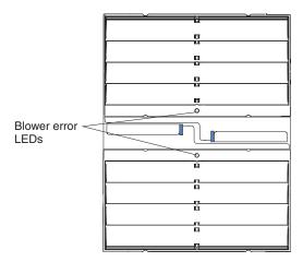
The LED on each blower provides status information about the blower. For additional information, see the Hardware Maintenance Manual and Troubleshooting Guide. This amber LED is lit and stays lit when an error has been detected in the blower. The system-error LEDs on the BladeCenter system LED panels are also lit.
