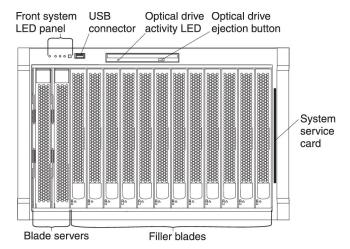
• Front system LED panel: The LEDs on this panel provide status information for your BladeCenter unit.
