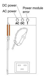
Power module LEDs: These LEDs indicate the condition of the power module.
