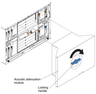
To install an acoustic attenuation module on the BladeCenter unit, complete the following steps:
