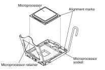
e. Center the microprocessor over the microprocessor socket. Align the triangle on the corner of the microprocessor with the triangle on the corner of the socket and carefully place the microprocessor into the socket.
