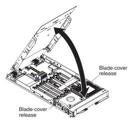
**Attention:** You cannot insert the blade server into the BladeCenter unit until the cover is installed and closed. Do not attempt to override this protection.
