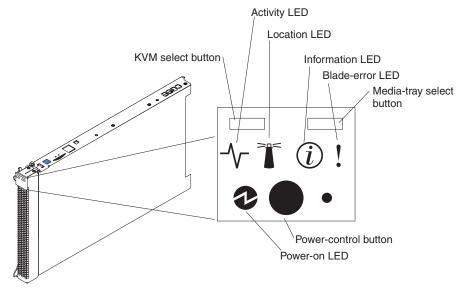
**Keyboard/video/mouse (KVM) select button:** Press this button to associate the shared BladeCenter unit keyboard port, video port, and mouse port with the blade server. The LED on this button flashes while the request is being processed, and then is lit when the ownership of the keyboard, video, and mouse has been transferred to the blade server. It can take approximately 20 seconds to switch the keyboard, video, and mouse control to the blade server.
