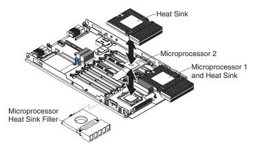
**Attention:** Do not touch the contacts in the microprocessor socket. Touching these contacts might result in permanent damage to the system board.
