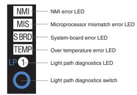
When you press the light path diagnostics switch, note which LEDs are lit on the system board and light path diagnostics panel. Using this information and the information in "Light path diagnostics LEDs" on page 93 can often provide enough information to diagnose the error.
