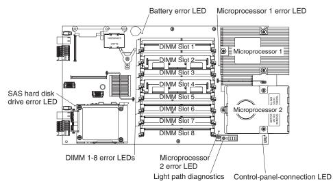
The following illustration shows LEDs on the system-board light path diagnostics panel.
