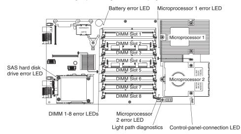
The following illustration shows the light path diagnostics panel on the system board.
