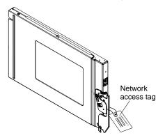
The front of the network access tag lists the CMM MAC address, default host name, and IPv6 link local address (LLA), as shown in the following illustration.
