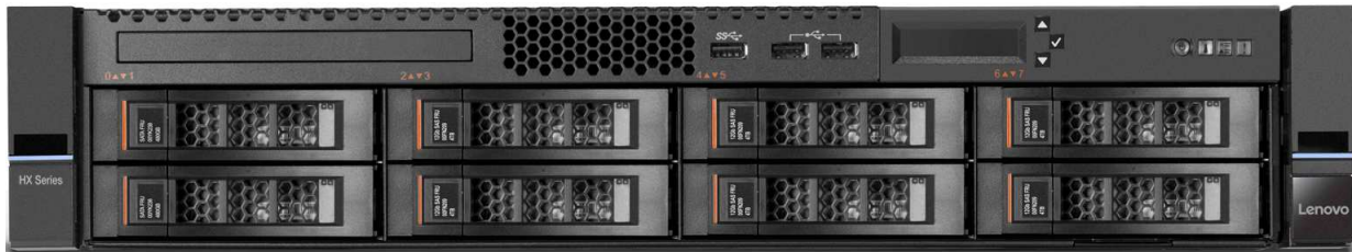
Figure 7. Front view HX5510 and HX5510-C eight 3.5-inch-drive configuration
