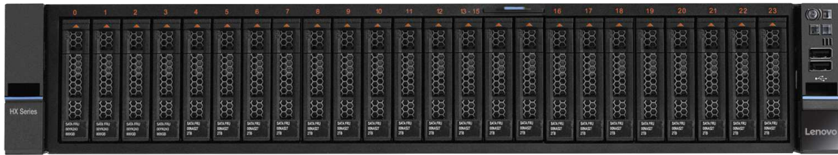
Figure 6. Front view HX7510 twenty-four 2.5-inch-drive configuration
