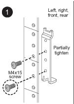
Do not install this screw on the front brackets for all 2U drive shelves and systems. It is installed after the equipment is in place.
