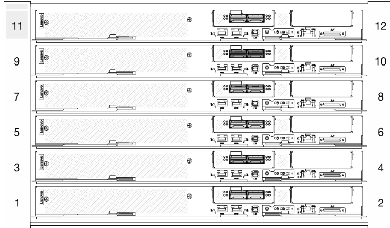
Figure 10. DW612S enclosure with six SD665-N V3 server
