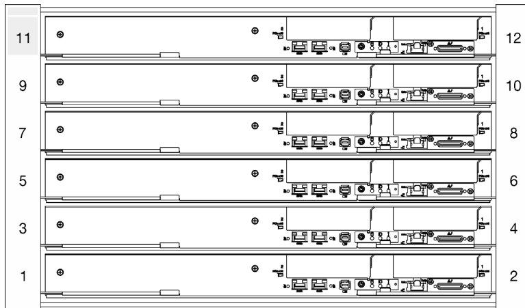
Figure 7. DW612S enclosure with six SD650-I V3 server
