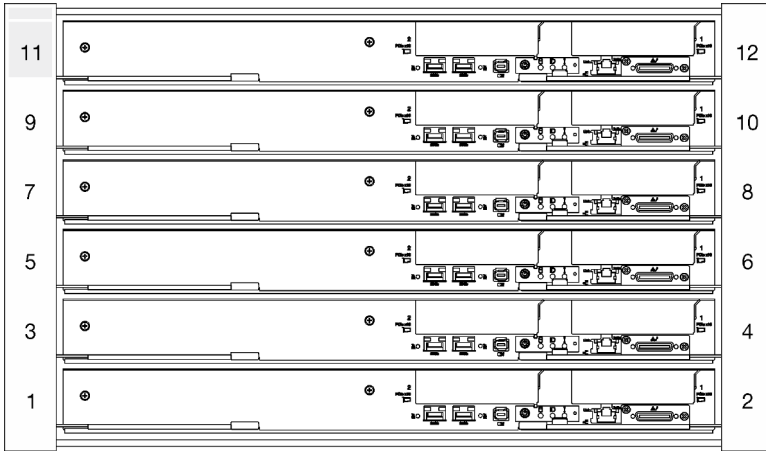
Figure 12. Enclosure with six SD650-I V3 trays
