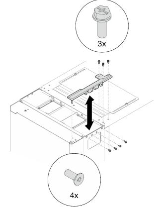
Figure 66. Installing the top hinge
