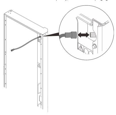
Figure 50. Removing the air-purging tool extension hose
