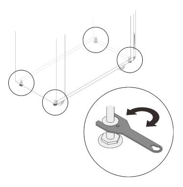
Figure 10. Lowering the leveling pads
