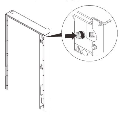
Figure 71. Installing the valve cap
