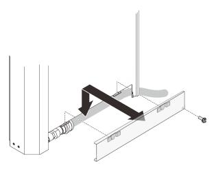
Figure 44. Removing the outer hose access pane
