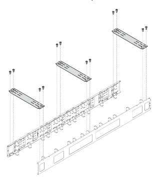
Figure 57. Removing the support brackets
