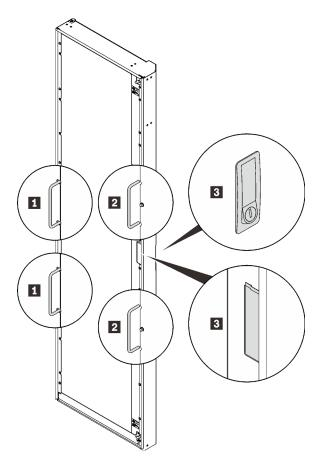
Figure 24. Lifting the heat exchanger with three people
