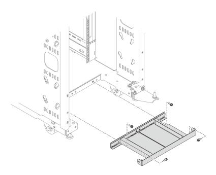
Figure 16. Installing the lower air baffle
