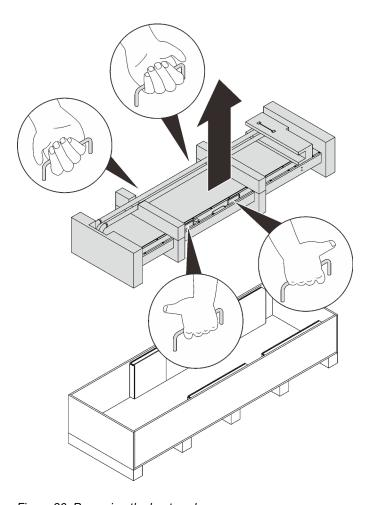
Figure 20. Removing the heat exchanger
