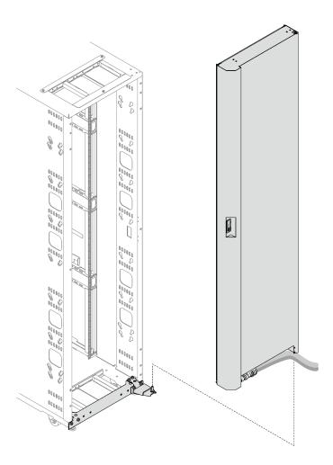
Figure 56. Removing the heat exchanger from the rack cabinet
