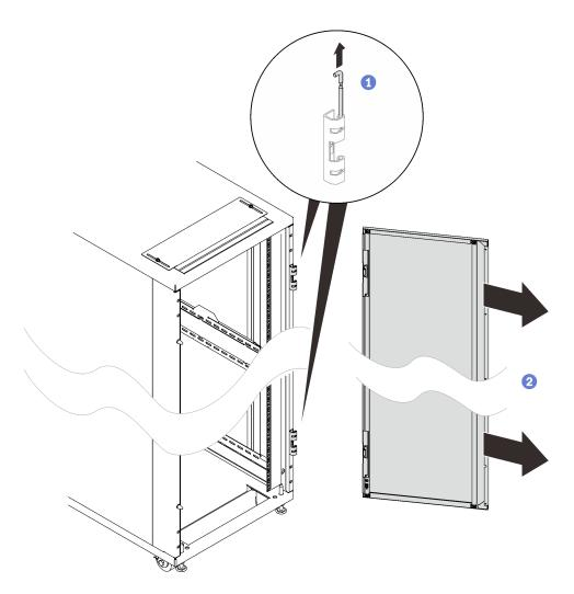
Figure 11. Removing a door
