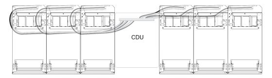
Figure 42. Routing and securing the hoses in raised-floor and non-raised-floor environments (from the top, looking down)
