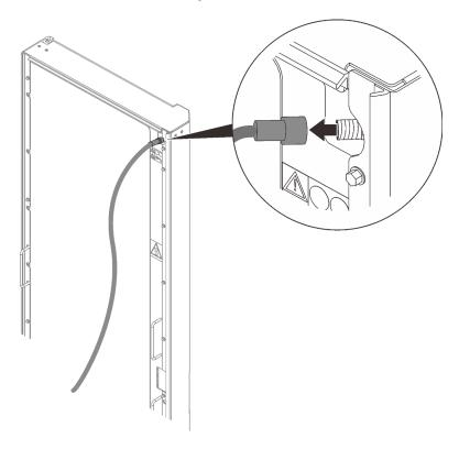
Figure 36. Removing the air-purging tool
