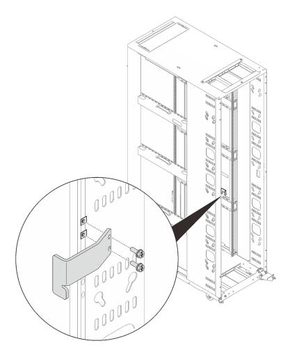
Figure 18. Installing the latch plate
