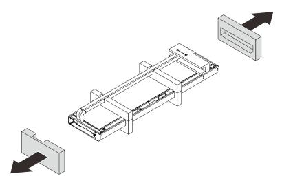
Figure 21. Removing the packing materials
