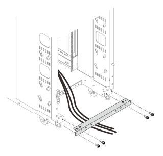
Figure 15. Removing the cable access bar
