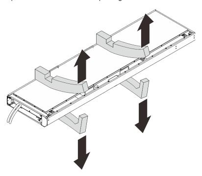
Figure 23. Removing the packing materials
