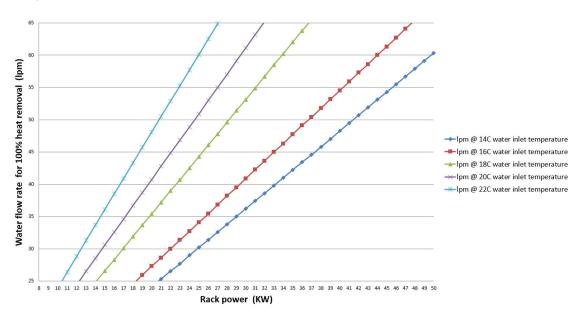
Figure 4. Typical performance of the heat exchanger, 4800SCFM Rack air flow, 25°C Rack entering temperature
