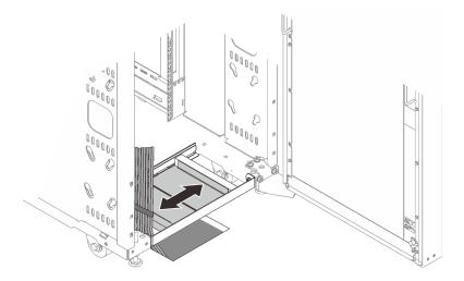
Figure 39. Managing cables with the lower air baffle
