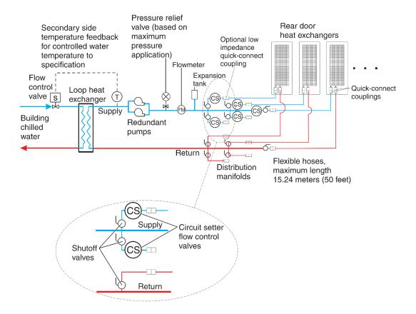
Figure 28. Coolant distribution unit with a fabricated facilities solution
