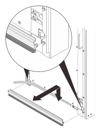
Figure 43. Removing the inner hose access panel
