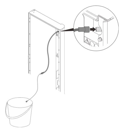
Figure 68. Installing the air-purging tool
