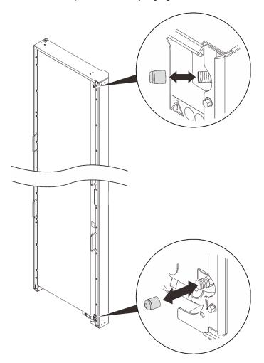
Figure 46. Removing valve caps
