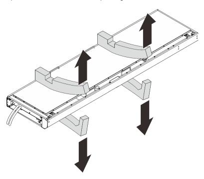
Figure 62. Removing the packing materials
