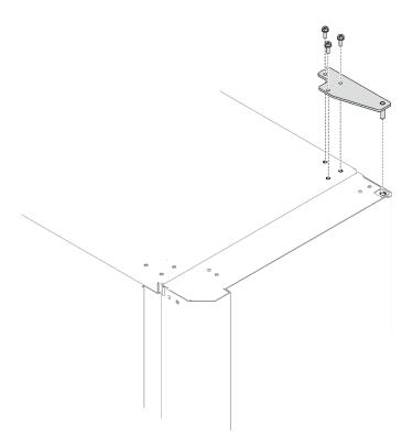
Figure 65. Installing the top hinge
