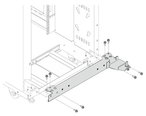
Figure 17. Installing the bottom hinge assembly
