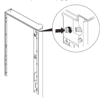
Figure 37. Installing the valve cap
