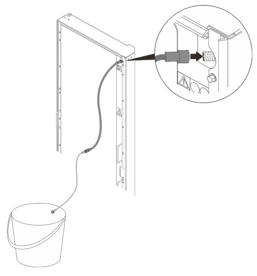
Figure 34. Installing the air-purging tool
