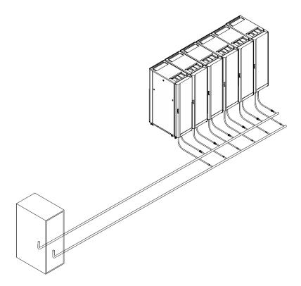
Figure 32. Typical extended manifold (along aisles between racks)
