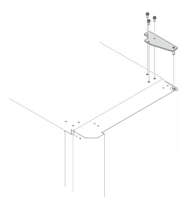
Figure 53. Removing the top hinge
