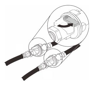
Figure 45. Opening Eaton ball valves
