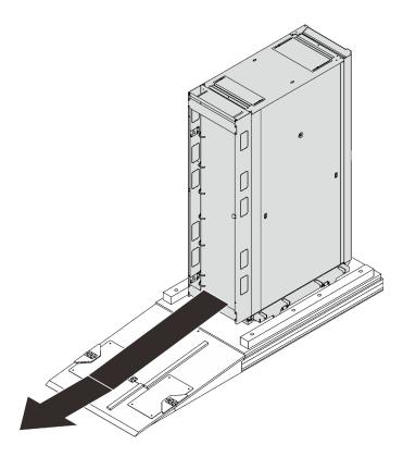
Figure 6. Moving the rack cabinet from the pallet
