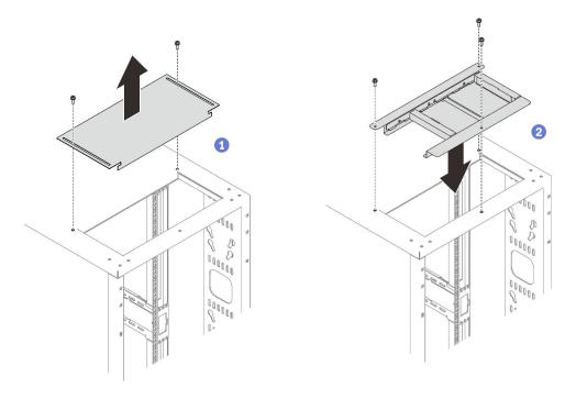
Figure 14. Installing the upper air baffle
