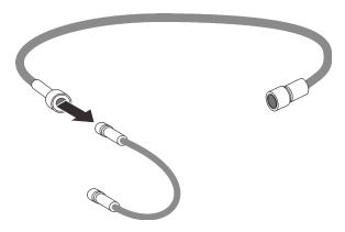
Figure 47. Removing the extension hose
