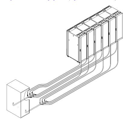
Figure 31. Typical central manifold (at a central location for multiple water circuits)
