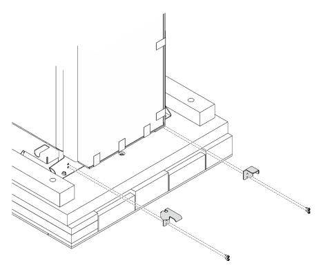
Figure 5. Removing the supporting brackets
