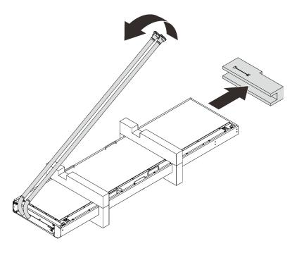
Figure 61. Removing the retaining material
