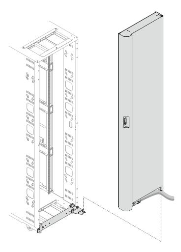
Figure 64. Installing the heat exchanger to the rack cabinet
