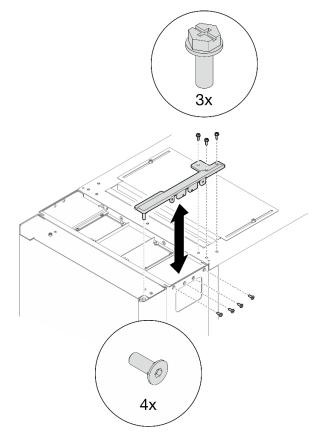
Figure 54. Removing the top hinge
