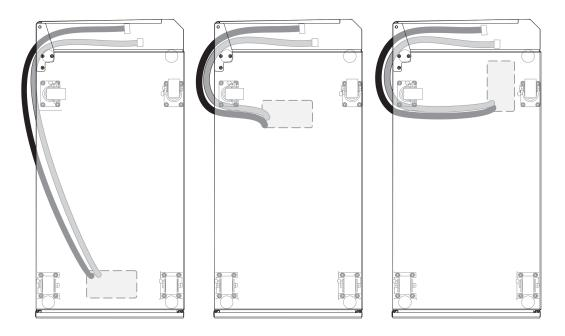
Figure 40. Routing and securing the hoses in a raised-floor environment for individual racks (from the top, looking down)
