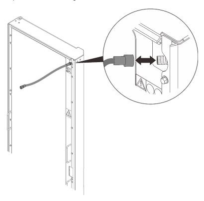
Figure 48. Inserting the air-purging tool extension hose
