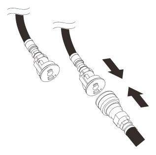
Figure 69. Connecting manifolds
