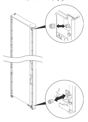
Figure 52. Installing the valve caps
