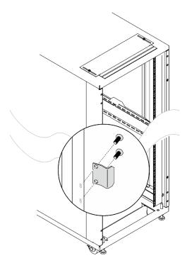
Figure 13. Removing the door latch
