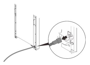
Figure 51. Removing the air-purging tool
