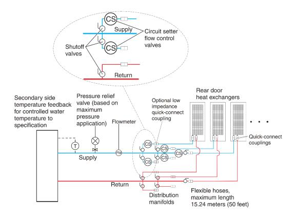
Figure 30. Coolant distribution unit that uses off-the-shelf supplier solutions
