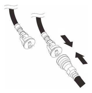
Figure 35. Connecting manifolds
