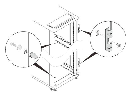
Figure 12. Removing the door hinges and doorstops
