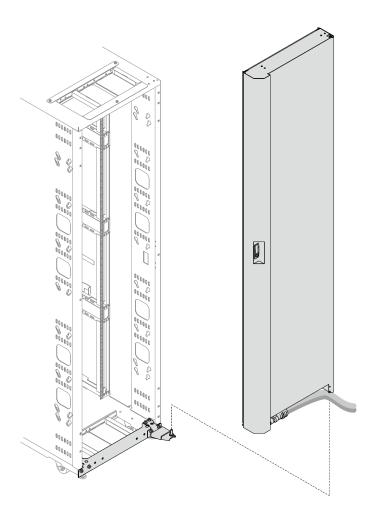
Figure 25. Installing the heat exchanger to the rack cabinet
