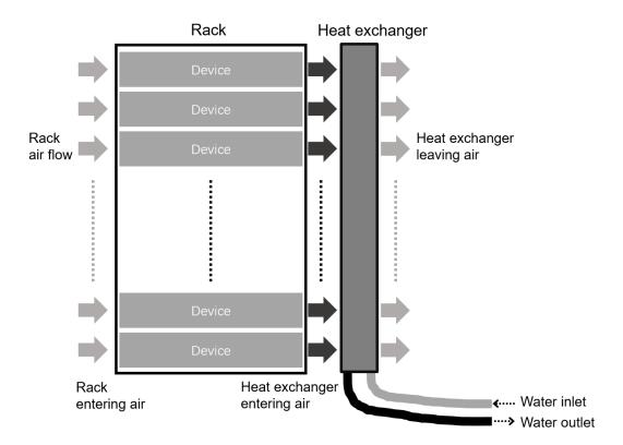
Figure 2. Diagram of rack air flow and heat exchanger water flow
