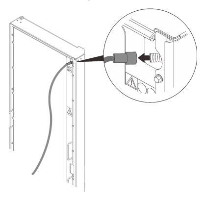
Figure 70. Removing the air-purging tool
