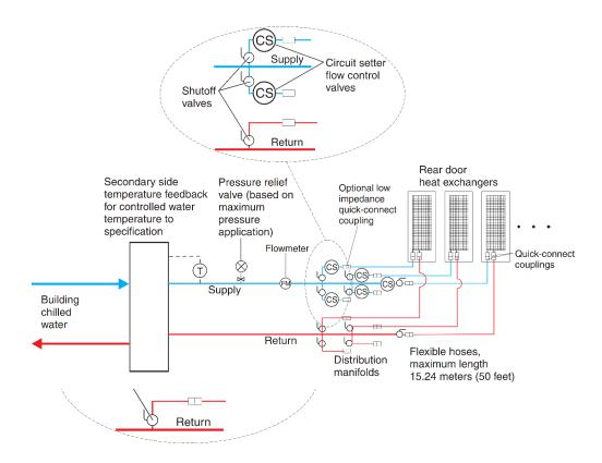
Figure 29. Coolant distribution unit that uses off-the-shelf supplier solutions
