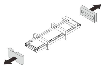
Figure 60. Removing the packing materials
