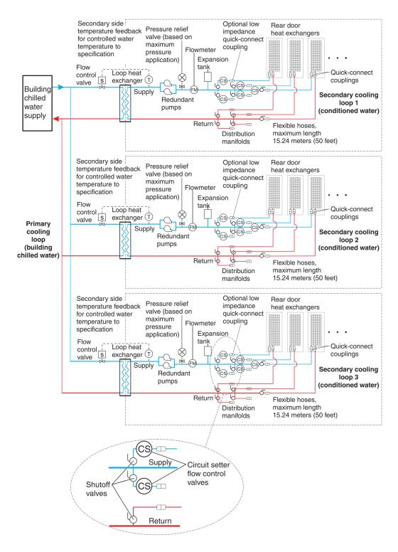
Figure 27. Primary and secondary cooling loops
