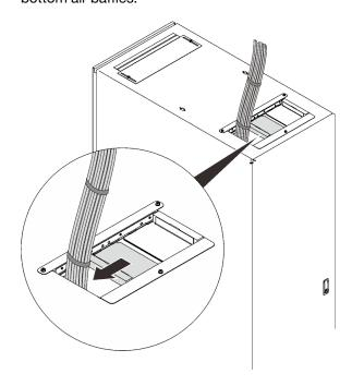
Figure 38. Managing cables with the upper air baffle
