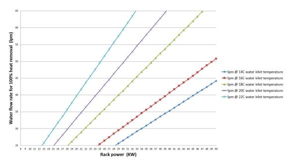
Figure 3. Typical performance of the heat exchanger, 3840SCFM Rack air flow, 25°C Rack entering temperature
