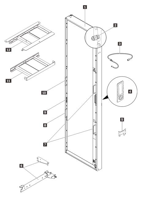
Figure 1. ThinkSystem Rear Door Heat eXchanger for 48U Rack components
