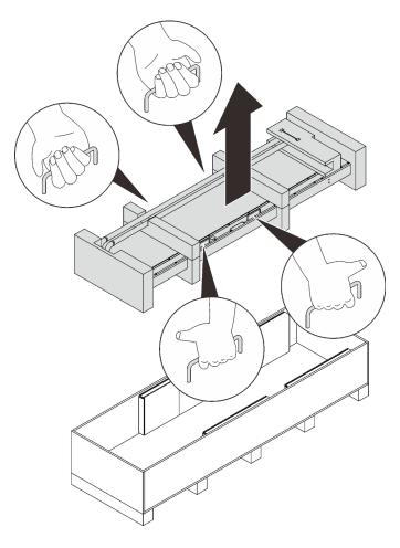
Figure 59. Removing the heat exchanger
