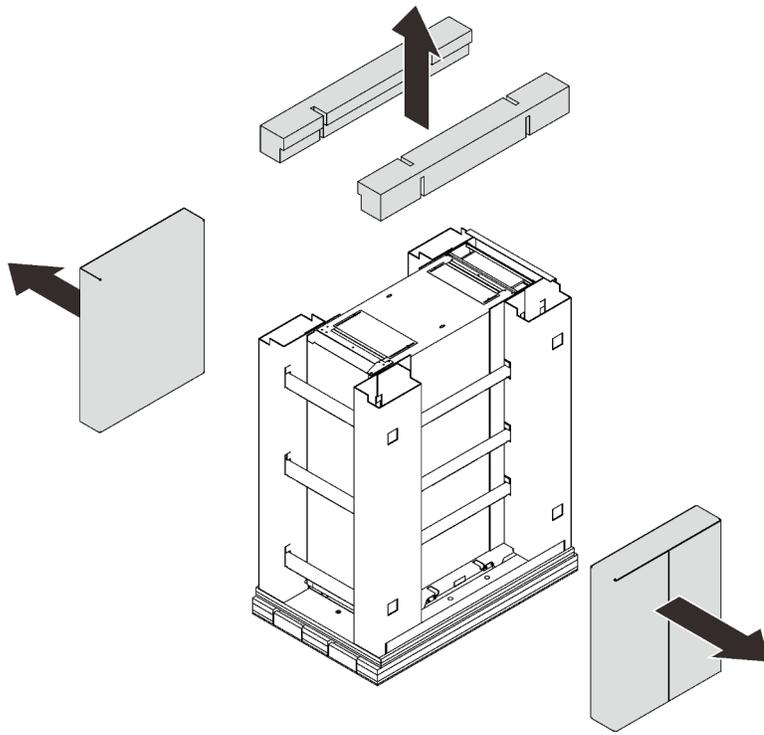
*Figura 4. Removendo as barras superiores e as caixas laterais*
