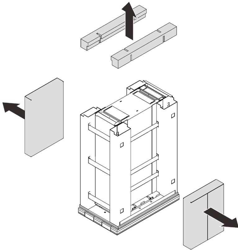
*Figura 4. Removendo as barras superiores e as caixas laterais*
