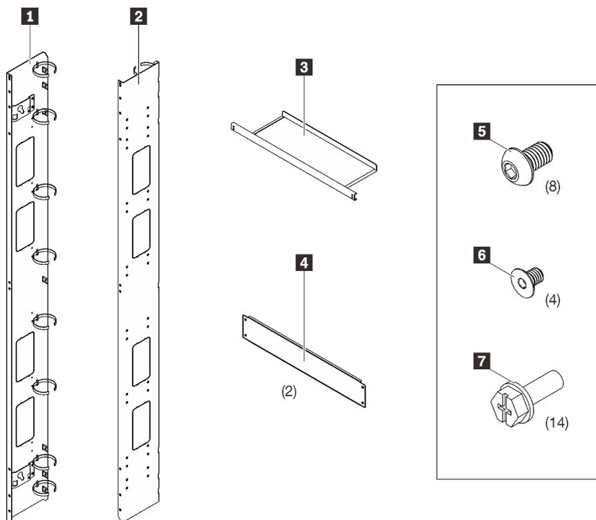
Рис. 6. 42U Standard Rack Extension Kit
