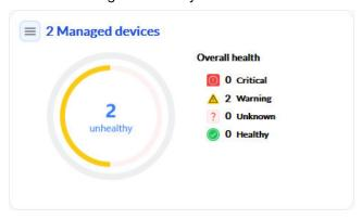
Click the Managed devices title to display the list of all managed devices, or click on a severity to display a filtered list of devices with that overall severity. The Managed devices page contains context menus for additional information.
