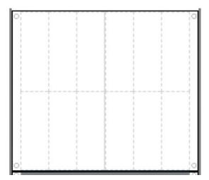
After that, you may set the blade location in the chassis. The row location (Start Grid X) is from left to right and the column location (Start Grid Y) is from bottom to top. For example, if one full-height blade is on the far right of the above chassis. Its 'Start Grid X' should be 6, 'Start Grid Y' should be 1, 'Width in Grids' should be 1 and 'Height in Grids' should be 2. Then it is shown like below.
