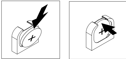
Figure 55. System battery installation
