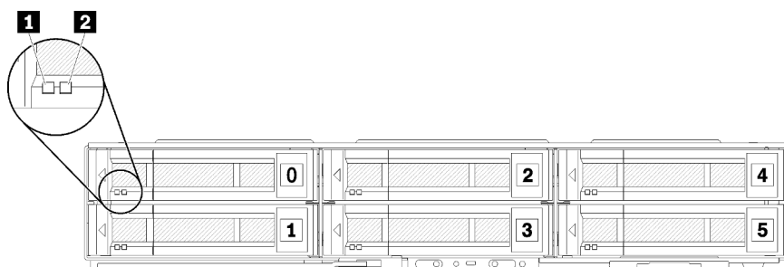
Figure 18. Six 2.5-inch drive configuration and drive bay numbering
