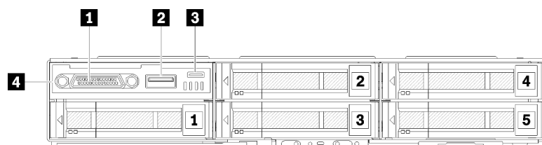
Figure 19. Five 2.5-inch drive configuration with KVM breakout module and drive bay numbering
