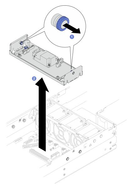
Figure 76. Removal of the internal adapter bracket
