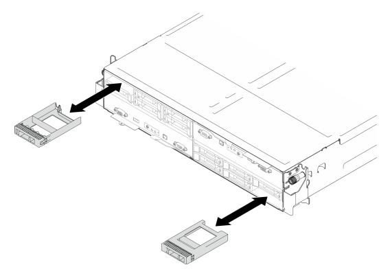
Figure 72. Replacement of a drive filler
