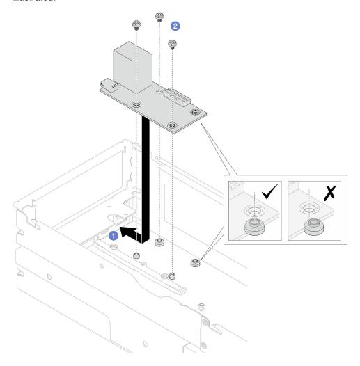
Figure 119. Installation of the rear I/O module
