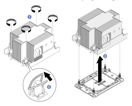
Figure 107. Removal of the 2U Standard PHM
