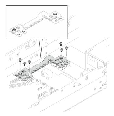
Figure 100. Removal of outer screws of the power bus bar
