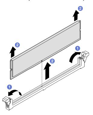
Figure 84. Removal of a memory module
