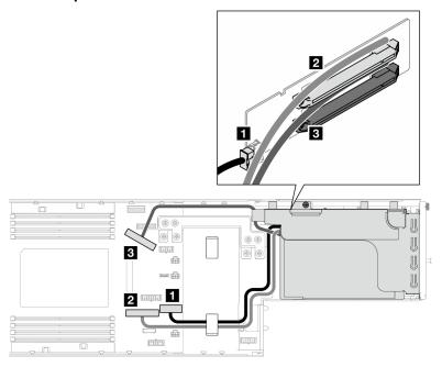
Figure 156. PCle riser cable routing – two processors
