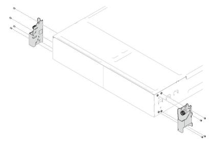
Figure 23. Installation of the EIA brackets
