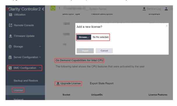
Figure 162. Uploading Activation Key via XCC Web GUI
