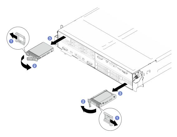
Figure 71. Removal of a 15mm solid-state drive
