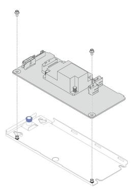
Figure 46. Separation of internal CFF RAID adapter from tray
