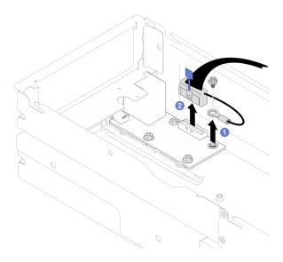
Figure 117. Removal of the rear I/O cable and grounding cable
