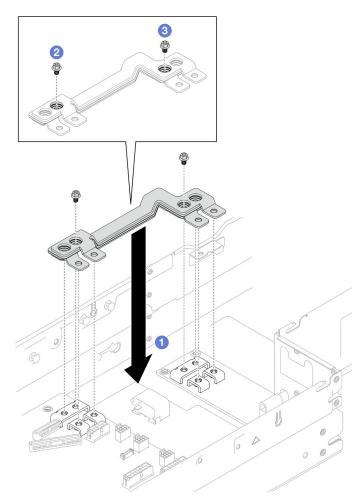
Figure 102. Installation of the power bus bar
