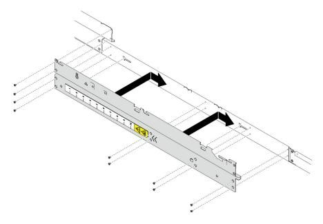
Figure 122. Installation of the side bracket
