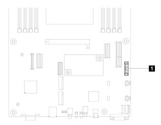
Figure 48. Location of the CMOS battery socket
