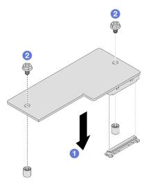
Figure 126. Installation of the firmware and RoT security module
