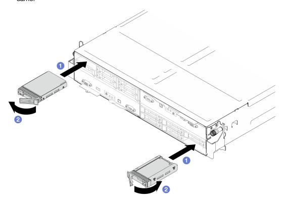
Figure 74. Installation of a 7mm solid-state drive
