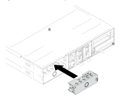
Figure 36. Installation of a rear node tray filler
