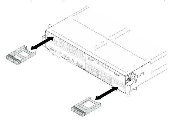
Figure 73. Replacement of a drive filler
