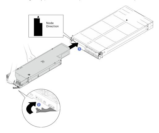
Figure 39. Node installation to the left tray
