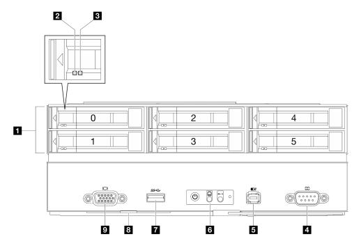
Figure 2. Configuration with up to six 2.5-inch drives
