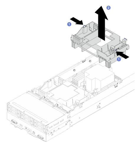
Figure 42. Removal of the rear air baffle
