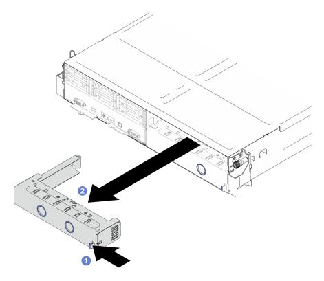
Figure 37. Removal of a front node tray filler
