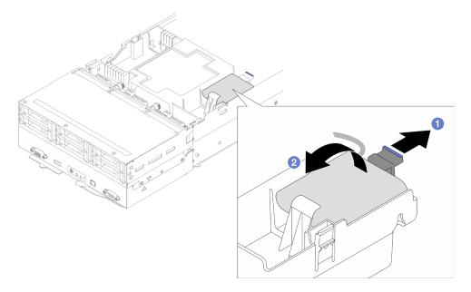
Figure 60. Removal of the flash power module
