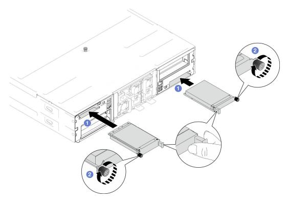
Figure 92. Installation of rear OCP module
