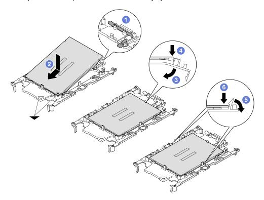
Figure 112. Installation of the processor carrier
