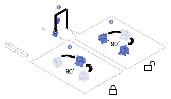
Figure 80. Adjustment of an M.2 drive retainer
