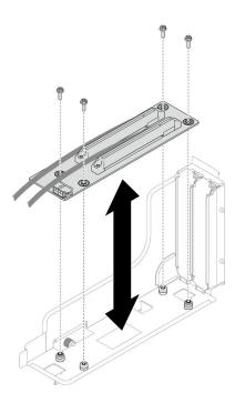
Figure 94. Replacement of the PCIe riser card
