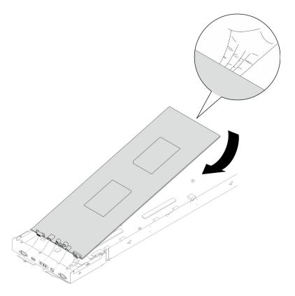
Figure 131. Installation of the system board
