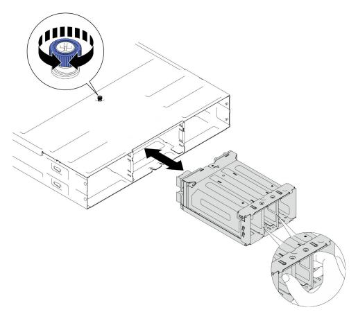
Figure 29. Removal of the PSU cage
