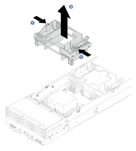
Figure 41. Removal of the front air baffle
