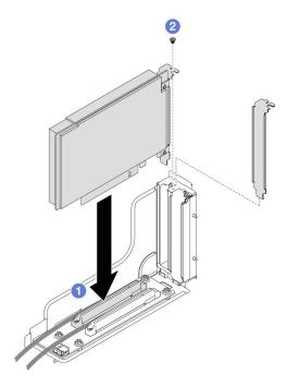
Figure 97. Installation of a PCIe adapter
