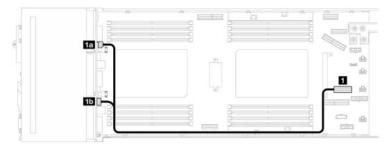
Figure 144. Drive backplane power cable routing
