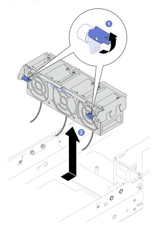
Figure 56. Removal of the fan cage
