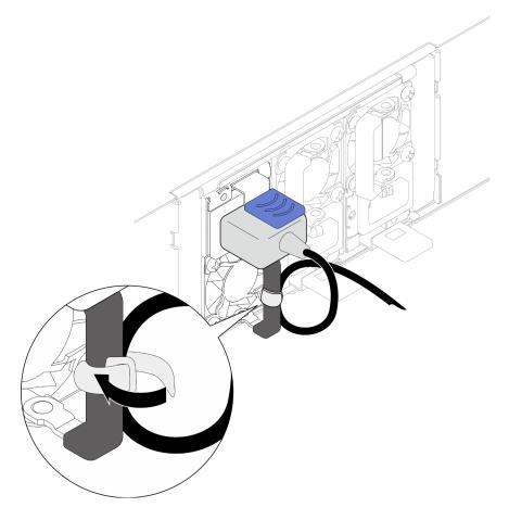
Figure 28. Routing and tying power cord
