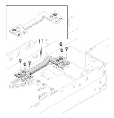
Figure 103. Installation of the power bus bar outer screws
