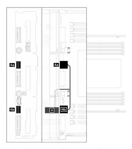
Figure 146. SATA cable routing- Configuration without CFF RAID
