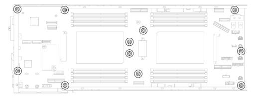
Figure 133. Installation of the screws on the system board
