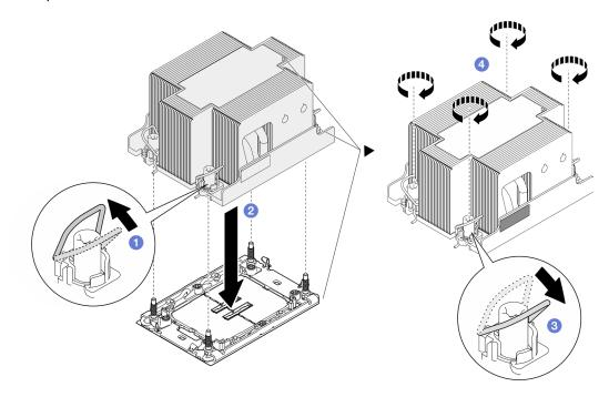
Figure 115. Installation of a 2U Standard PHM
