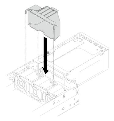
Figure 69. Installation of the GPU air duct
