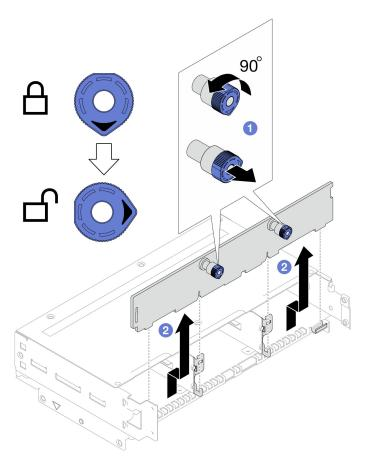
Figure 53. Removal of the drive backplane
