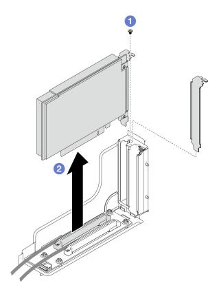
Figure 95. Removal of a PCIe adapter
