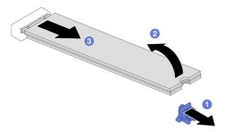
Figure 79. Removal of an M.2 drive
