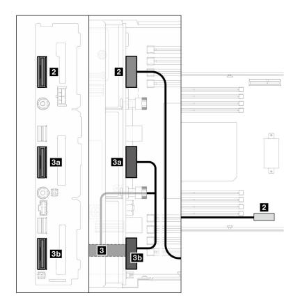
Figure 145. NVMe cable routing
