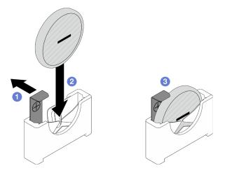
Figure 51. Installation of a CMOS battery
