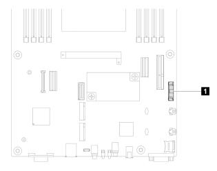
Figure 50. Location of the CMOS battery socket
