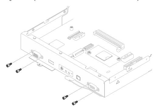
Figure 132. Installation of the system-board screws on the front
