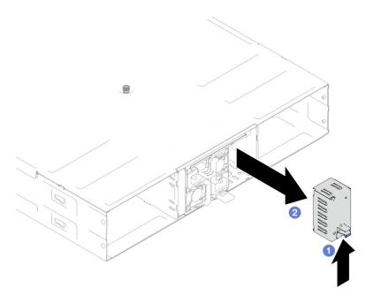
Figure 26. Removal of a PSU filler
