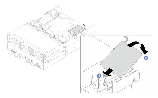
Figure 61. Installation of the flash power module
