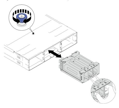
Figure 32. Installation of the PSU cage
