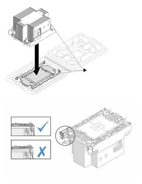
Figure 114. Assembling the PHM with processor in shipping tray
