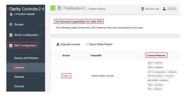
Figure 164. Checking the Intel On Demand features installed in a processor in XCC Web GUI
