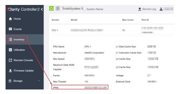
Figure 161. Reading PPIN via XCC Web GUI
