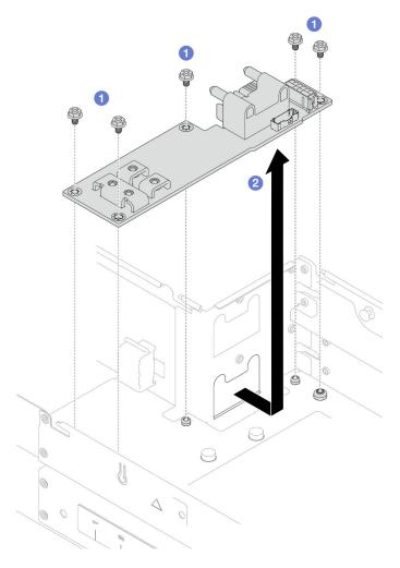
Figure 104. Removal of the power distribution board
