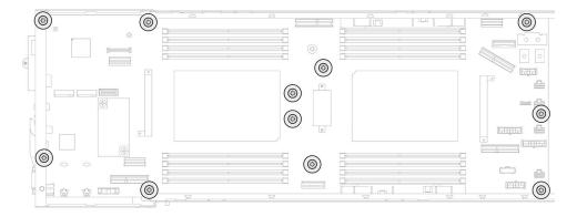
Figure 129. Removal of the screws
