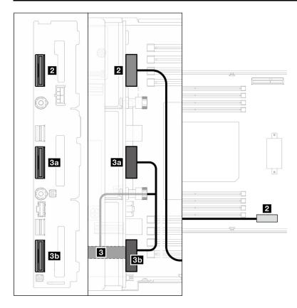
Figure 148. NVMe cable routing
