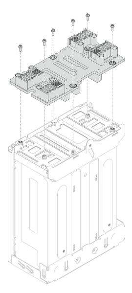
Figure 30. Removal of the chassis midplane
