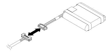
Figure 151. Flash power module extension cable
