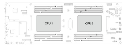
Figure 85. Memory module and processor location
