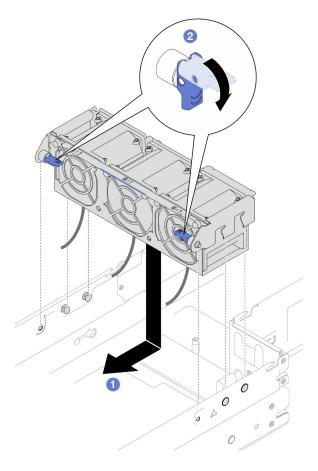
Figure 59. Installation of the fan cage
