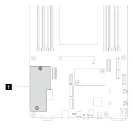
Figure 123. Location of the Firmware and RoT security module
