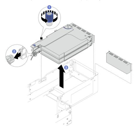
Figure 93. Removal of the PCIe riser assembly
