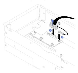
Figure 120. Installation of the rear I/O cable and grounding cable
