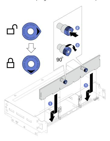
Figure 54. Installation of the drive backplane
