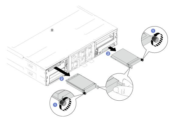
Figure 91. Removal of the rear OCP module
