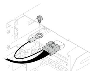
Figure 64. Screw of the front I/O grounding cable
