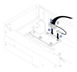
Figure 159. Installation of the rear I/O cable and grounding cable
