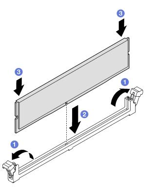
Figure 86. Installation of a memory module
