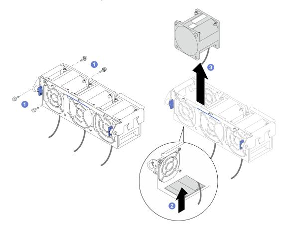
Figure 57. Fan removal
