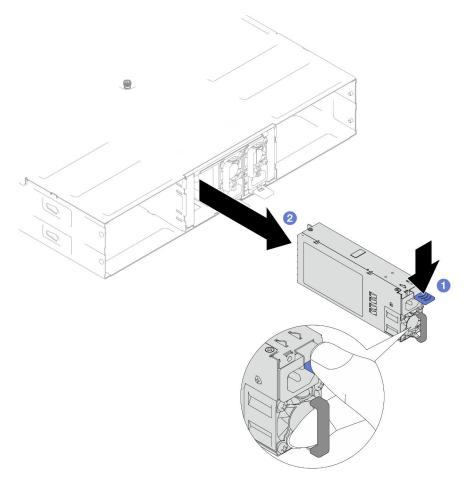
Figure 24. Removal of a hot-swap PSU
