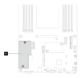
Figure 125. Location of the Firmware and RoT security module
