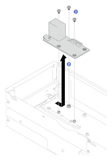
Figure 118. Removal of the rear I/O module
