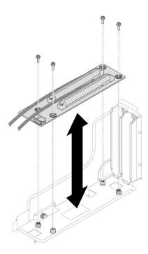
Figure 96. Replacement of the PCIe riser card
