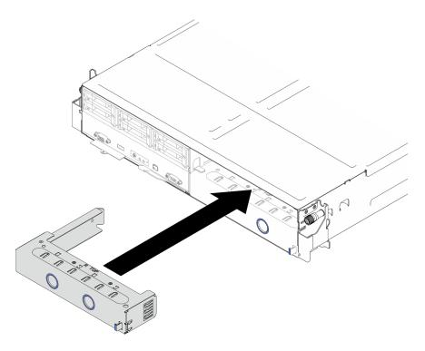
Figure 35. Installation of a front node tray filler
