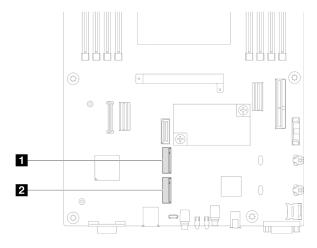
Figure 78. Location of the M.2 bays on the system board
