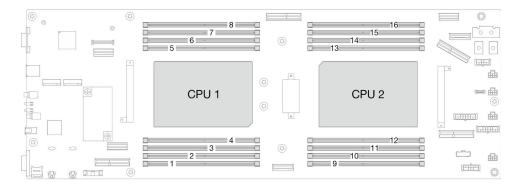
Figure 83. Memory module and processor location
