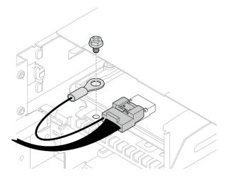
Figure 67. Screw of the front I/O grounding cable
