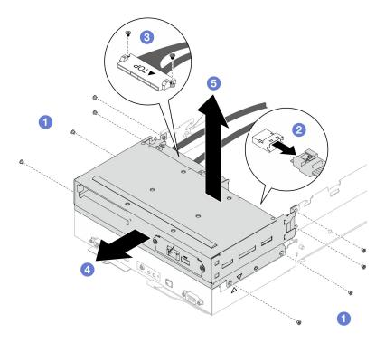
Figure 65. Removal of the front OCP cage
