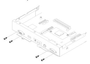
Figure 128. Removal of the screws
