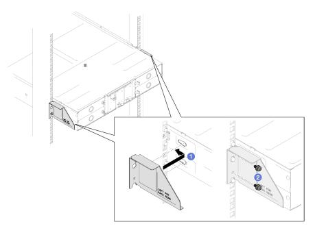
Figure 20. Installation of shipping brackets for 29-inch or 28.31-inch deep racks
