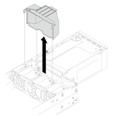
Figure 68. Removal of the GPU air duct
