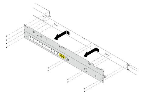
Figure 121. Removal of the side bracket
