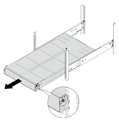
Figure 18. Chassis removal
