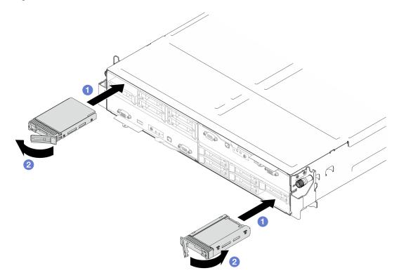
Figure 75. Installation of a 15mm solid-state drive
