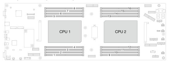
Figure 15. Memory modules and processors layout
