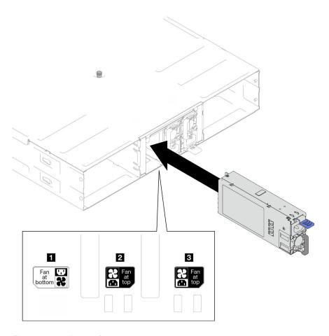
Figure 27. Installation of a hot-swap power supply
