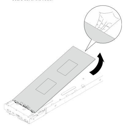
Figure 130. Removal of the system board
