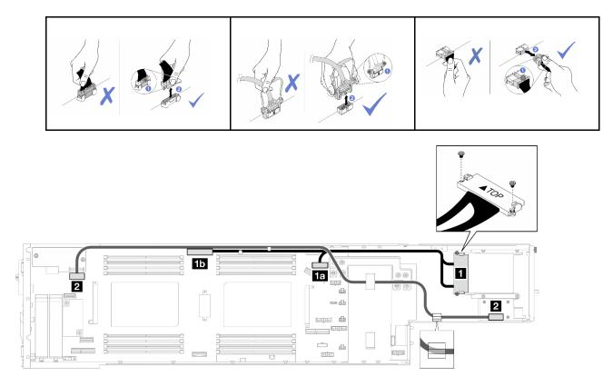
Figure 158. Cables for the rear I/O module and OCP module
