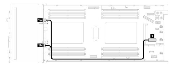
Figure 147. Drive backplane power cable routing
