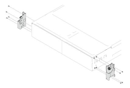
Figure 22. Removal of the EIA brackets
