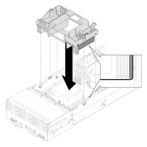
Figure 43. Installation of the front air baffle
