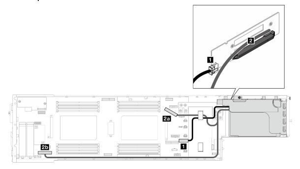
Figure 155. PCle riser cable routing – one processor
