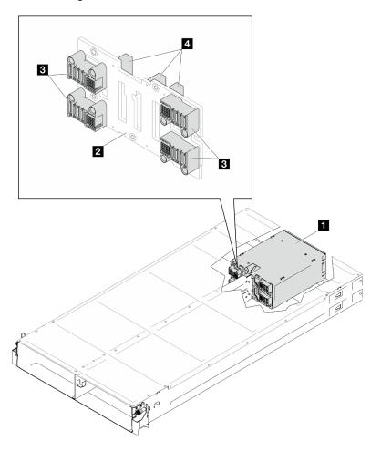
Figure 8. Chassis midplane location and connectors
