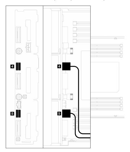
Figure 149. SATA cables on drive backplane
