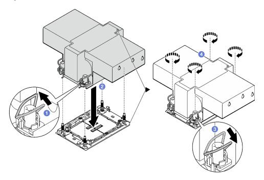
Figure 116. Installation of a 2U performance PHM
