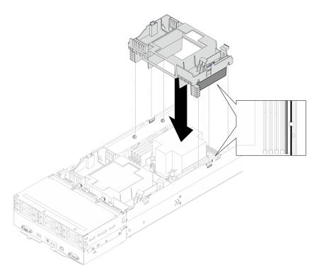
Figure 44. Installation of the rear air baffle
