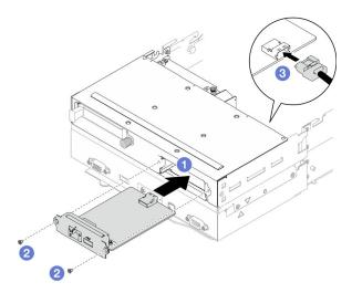
Figure 138. Installation of an XCC management module
