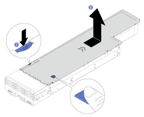
Figure 135. Removal of the top cover
