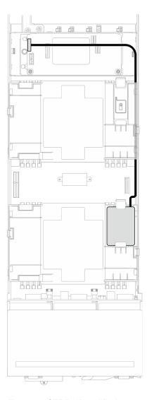
Figure 63. CFF RAID and flash power module cable
