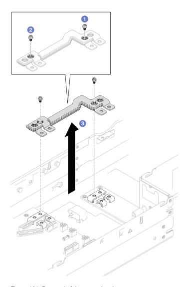
Figure 101. Removal of the power bus bar
