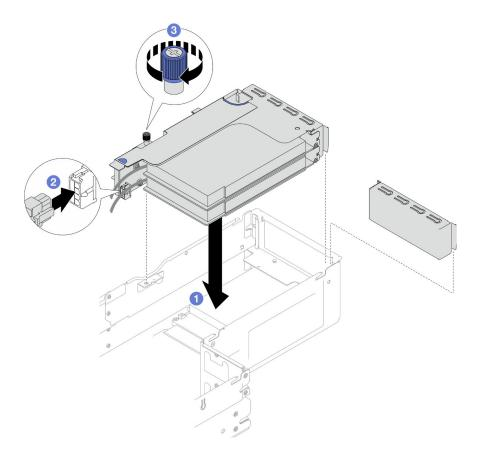
Figure 99. Installation of the PCle riser assembly
