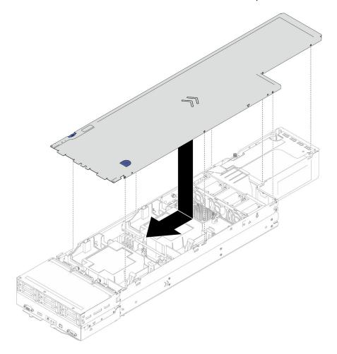
Figure 136. Installation of the top cover
