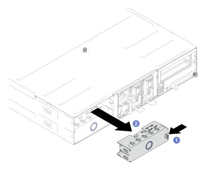
Figure 38. Removal of a rear node tray filler
