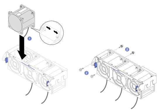
Figure 58. Fan installation
