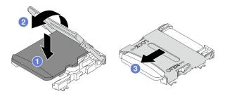
Figure 90. Installation of a MicroSD card
