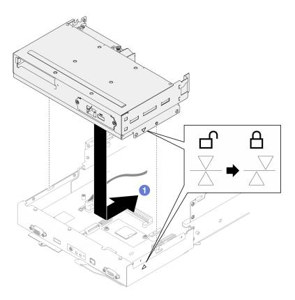
Figure 66. Installation of the front OCP cage
