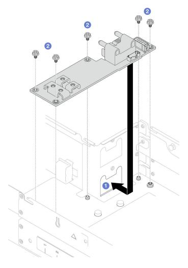
Figure 105. Installation of a power distribution board
