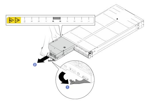
Figure 33. Node removal from the left tray
