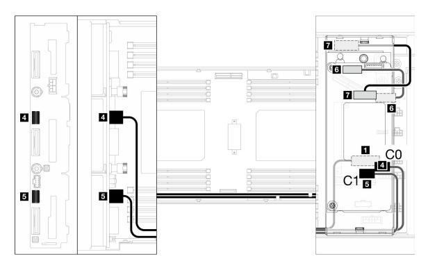
Figure 150. SATA and CFF RAID cable routing
