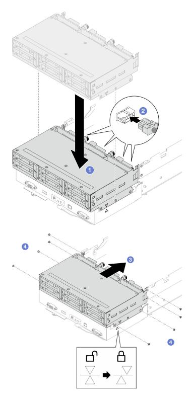
Figure 55. Installation of the drive cage assembly
