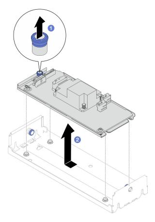
Figure 45. Removal of the internal CFF adapter
