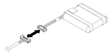
Figure 62. Flash power module extension cable
