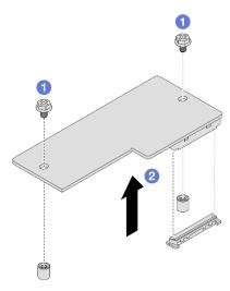
Figure 124. Removal of the Firmware and RoT security module
