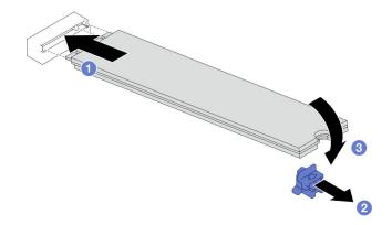
Figure 82. Installation of an M.2 drive
