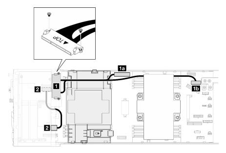
Figure 153. OCP cable and front I/O cable in the front OCP configuration
