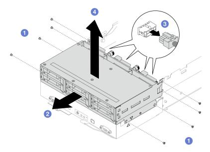
Figure 52. Removal of the drive cage assembly
