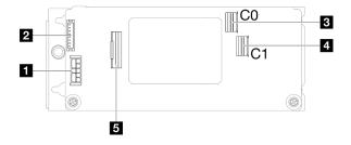
Figure 140. Internal CFF RAID adapter connectors
