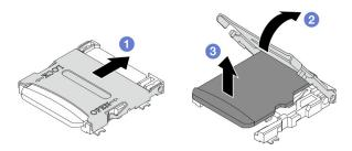
Figure 88. Removal of the MicroSD card
