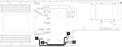
Figure 157. Cable routing for the power distribution board
