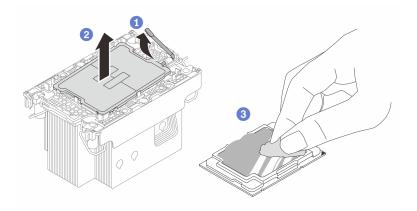
Figure 109. Separating a processor carrier from the heat sink
