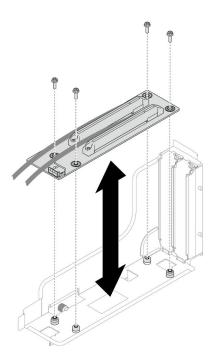
Figure 98. Replacement of the PCIe riser card
