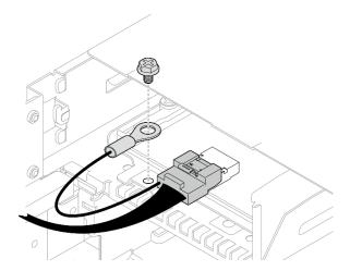
Figure 154. Screw of the front I/O grounding cable
