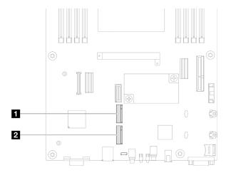
Figure 81. Location of the M.2 bays on the system board
