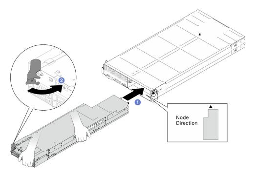
Figure 40. Node installation to the right tray
