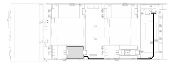
Figure 152. CFF RAID and flash power module cable
