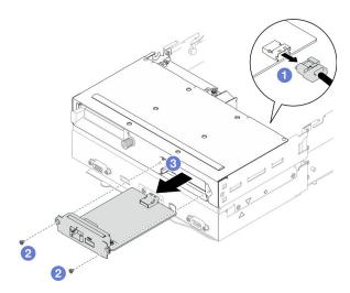
Figure 137. Removal of the XCC management module
