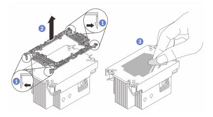
Figure 110. Separating a processor carrier from the heat sink
