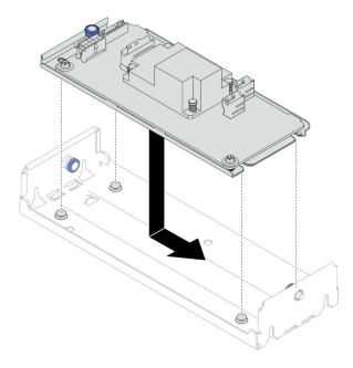
Figure 47. Installation of the internal CFF RAID adapter to the bracket
