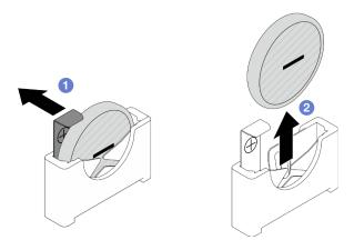
Figure 49. Removal of the CMOS battery
