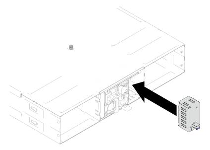
Figure 25. Installation of a PSU filler
