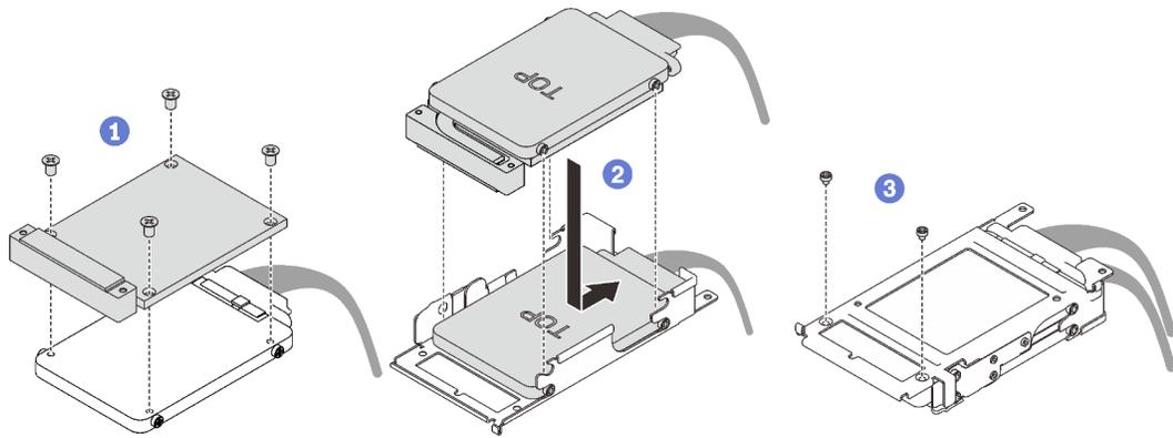
Figure 51. Upper drive installation
