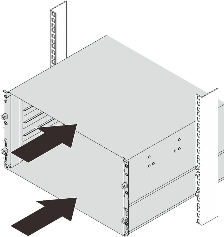
Figure 65. Sliding the rack
