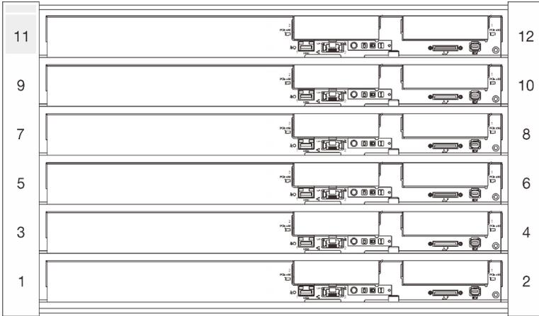
Figure 8. Enclosure with six SD650-N V2 trays
