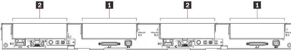
Figure 19. PCIe slot numbering - SD650 V2 tray
