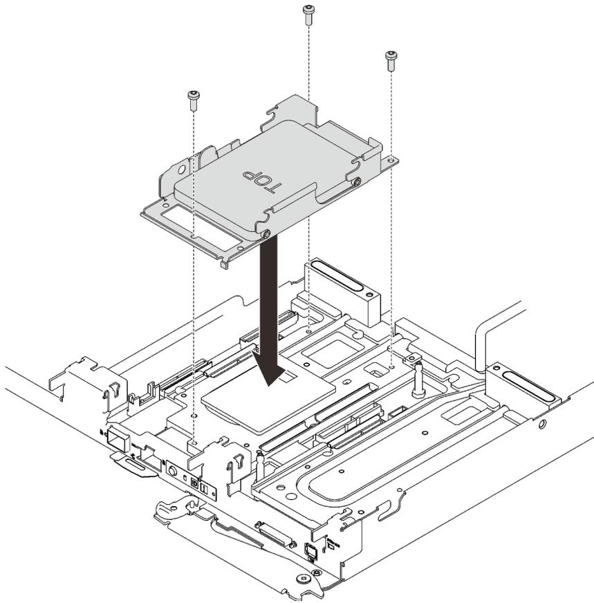
Figure 58. One-drive cage assembly installation
