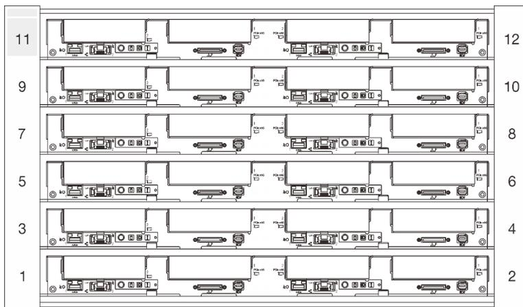
Figure 7. Enclosure with six SD650 V2 trays
