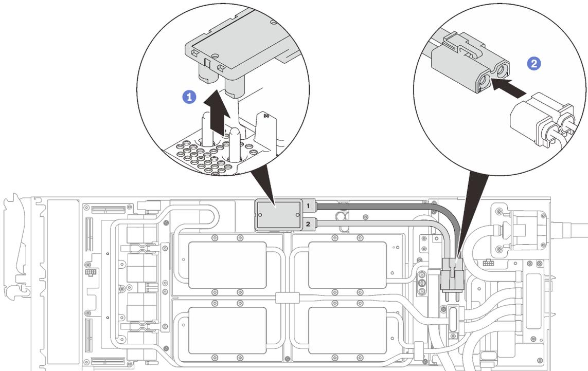
Figure 29. GPU power cable removal
