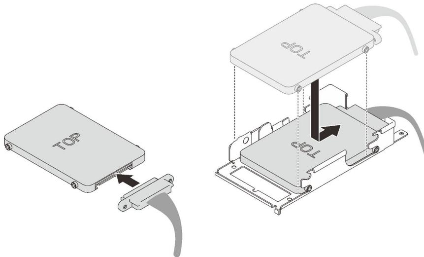
Figure 50. Lower drive installation
