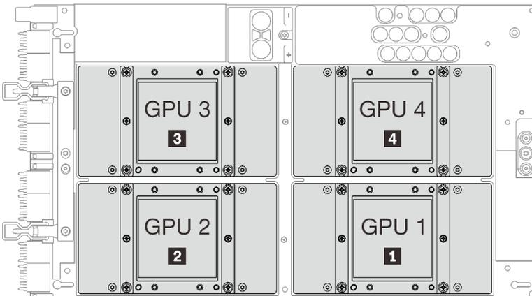
Figure 21. GPU numbering - SD650-N V2 tray
