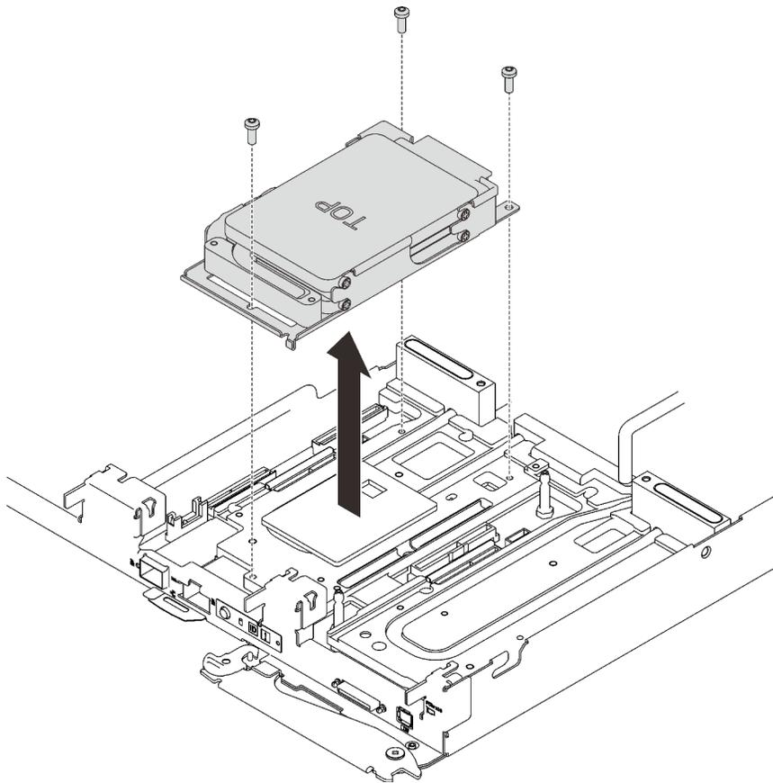
Figure 39. Two-drive cage assembly removal
