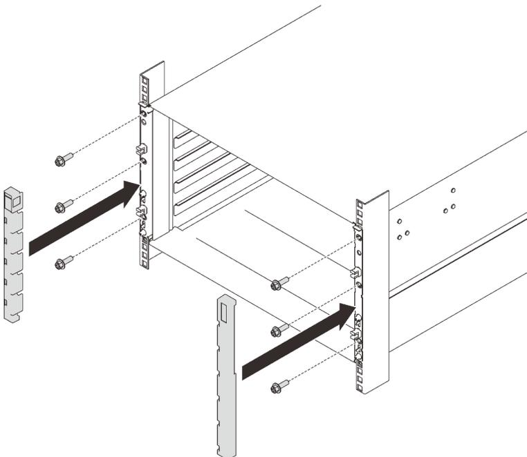
Figure 66. EIA cover installation
