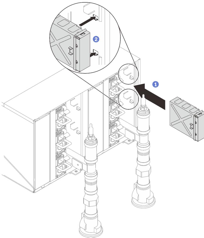
Figure 70. Blank filler installation
