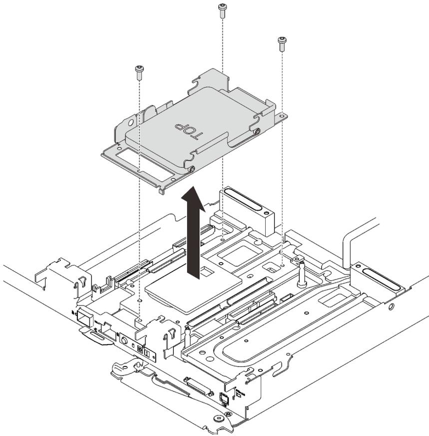
*Figure 38. One-drive cage assembly removal*
