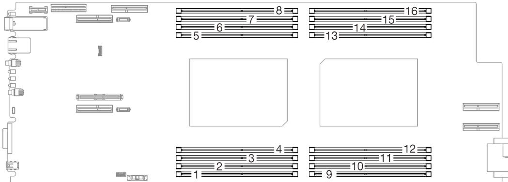
Figure 16. The location of the DIMM connectors on the system board of the compute node
