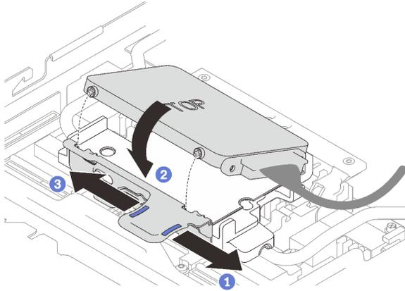
Figure 53. Drive cage installation
