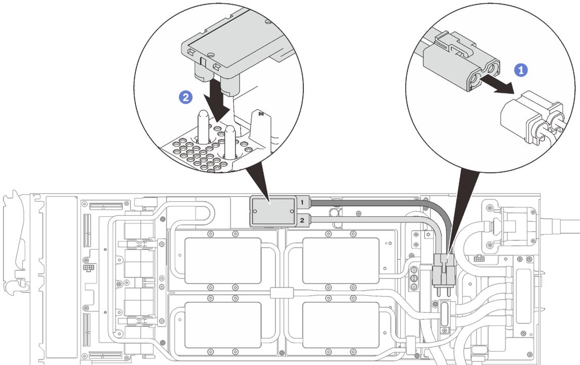
Figure 24. GPU power cable installation
