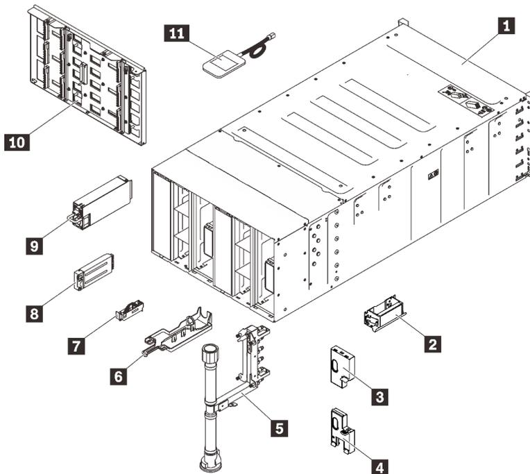
Figure 30. Enclosure components
