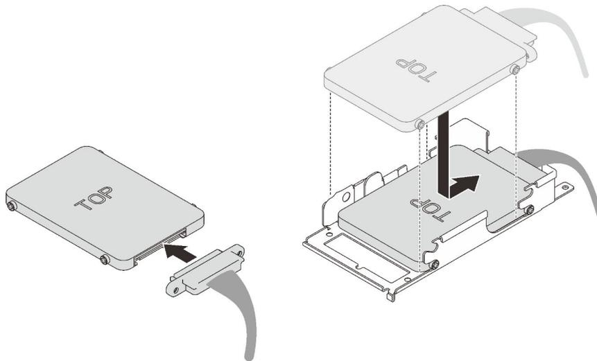
Figure 49. Drive installation
