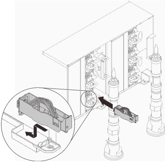
Figure 74. Drip sensor assembly installation
