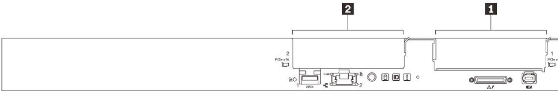
Figure 20. PCIe slot numbering - SD650-N V2 tray
