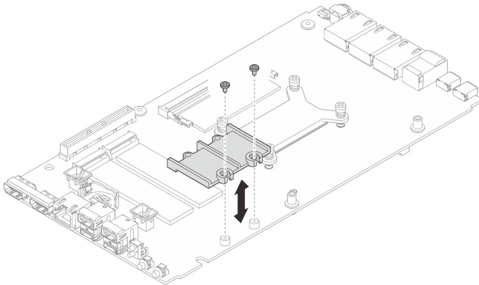
Figure 114. Installation du support M.2
