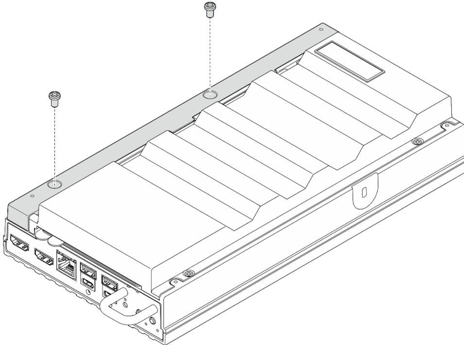
Figure 80. Installation des vis
