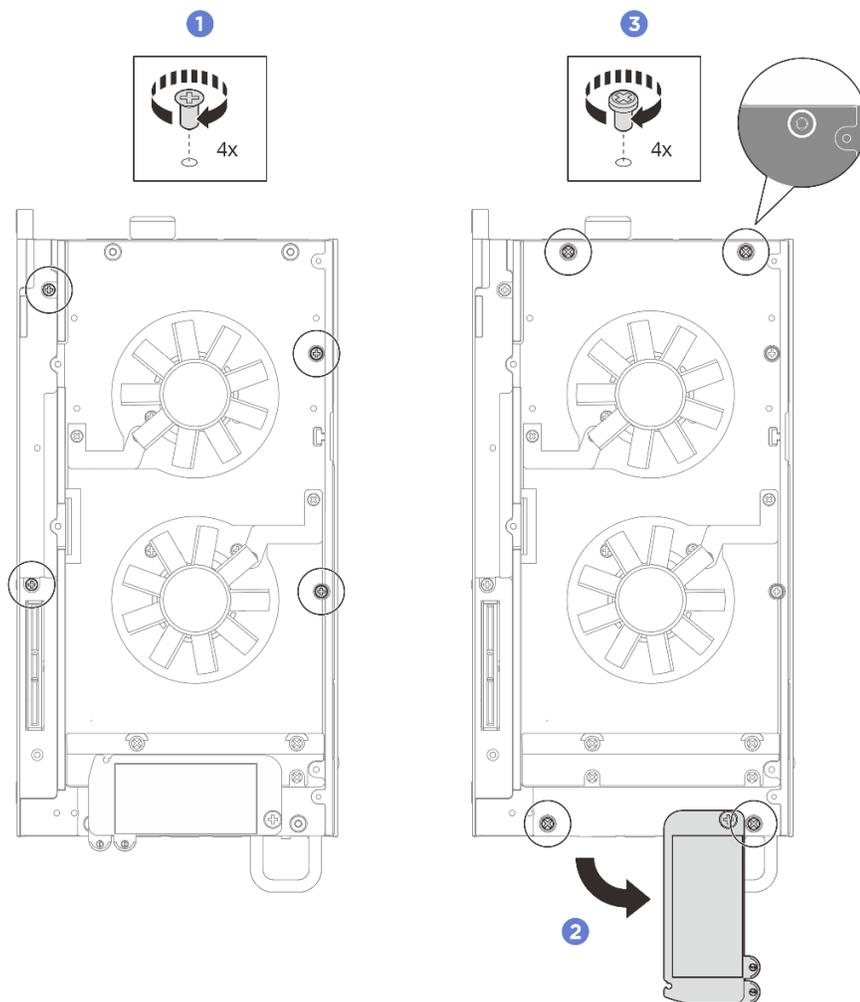
Figure 147. Installation des vis
