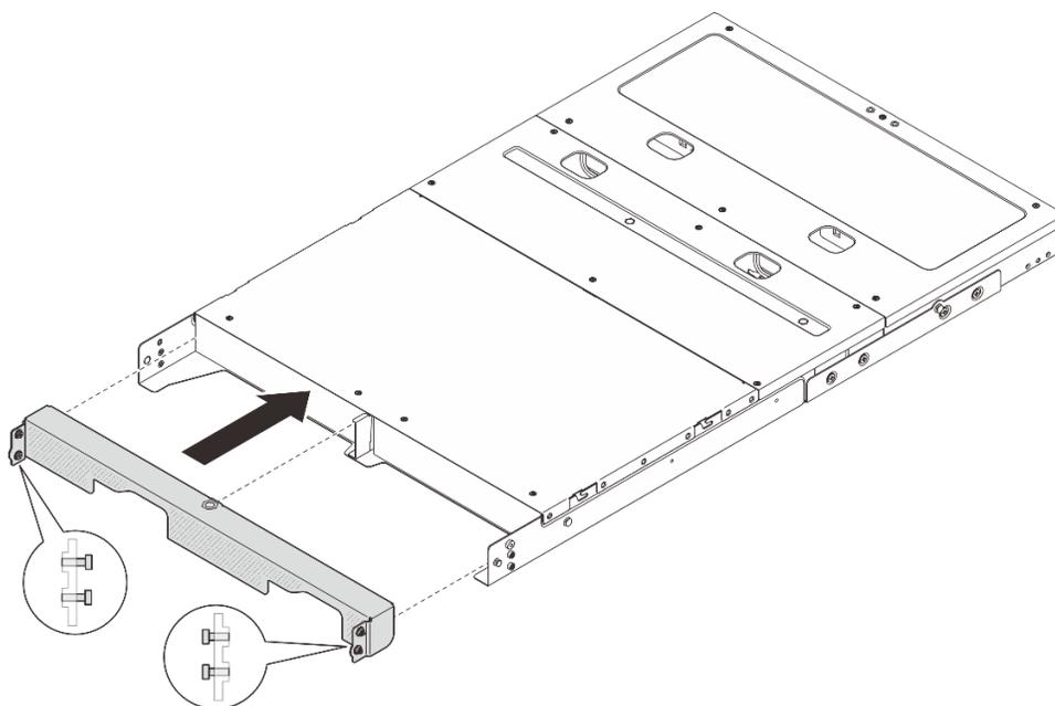
Figure 19. Installation du support de transport
