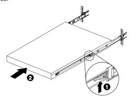
7. Secure the server before you move the rack, or if you place the rack in a vibration-prone area. Open the latches **1** in the front of the server, and then tighten the screws **2**.
