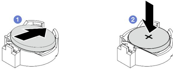
Figure 121. Installer la pile CMOS
