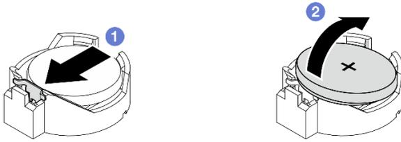
Figure 118. Retirer la pile CMOS
