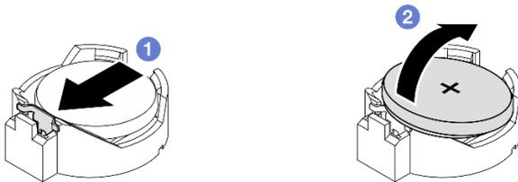
Figure 119. Retirer la pile CMOS
