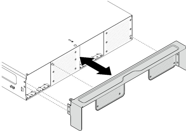
Figure 12. Installation du support de transport
