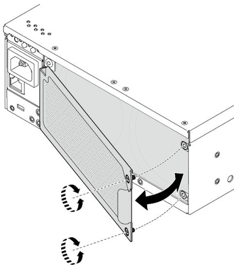
Figura 75. Instalando o painel
