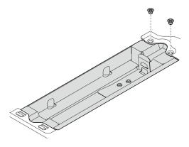
Figure 260. Installing the geotracking module cage
