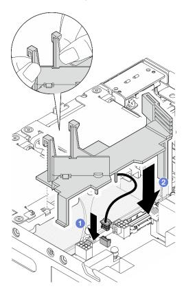
Figure 93. Installing the air baffle
