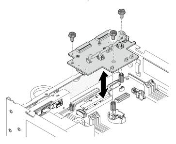
Figure 112. Installing the wireless adapter
