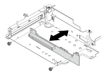
Figure 230. Removing the riser card
