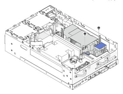
Figure 141. Fastening the screws
