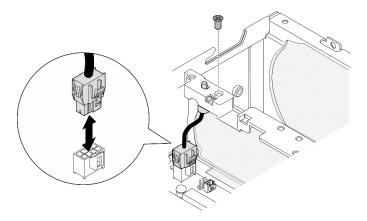
Figure 124. Removing the fan direction switch
