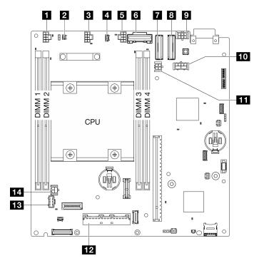
Figure 342. System-board connectors
