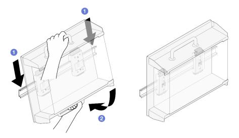
Figure 66. Installing the node sleeve
