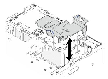
Figure 86. Removing the air baffle
