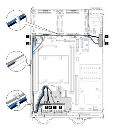
Figure 344. WLAN antenna cable routing
