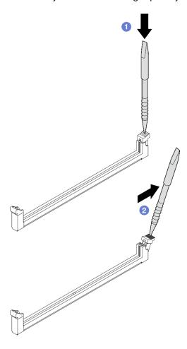
Figure 182. Opening retaining clip
