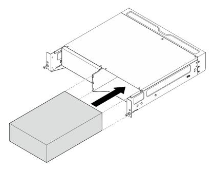
Figure 22. Installing the node
