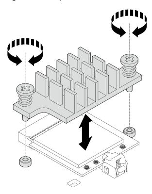
Figure 291. Installing the WLAN/Bluetooth module heat sink
