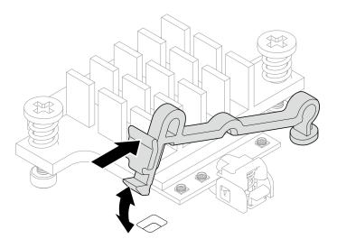
Figure 111. Inserting the cable holder
