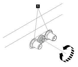
Figure 19. Shortening the SMA connectors
