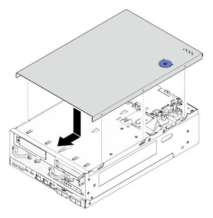
Figure 190. Installing the top cover
