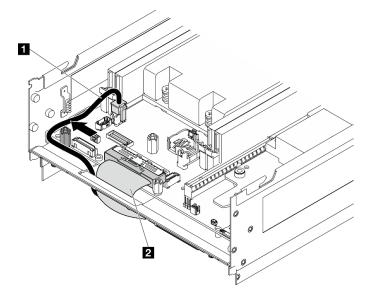
Figure 160. I/O-board cable routing
