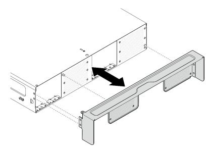
Figure 11. Removing the shipping bracket
