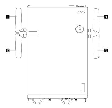
Figure 354. Locations of WLAN antennas
