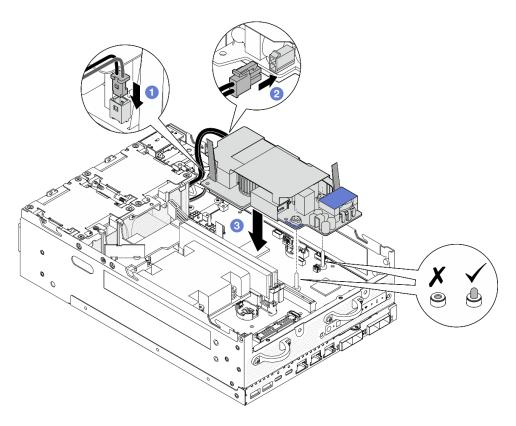
Figure 140. Installing the internal power supply unit
