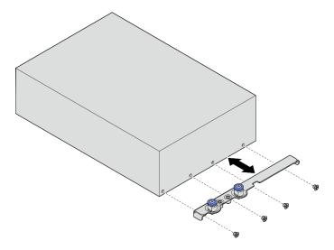
Figure 6. Removing the enclosure bracket
