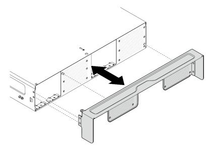
Figure 12. Installing the shipping bracket
