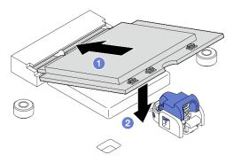
Figure 289. Installing the WLAN/Bluetooth module
