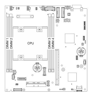
Figure 178. Memory modules and processor layout
