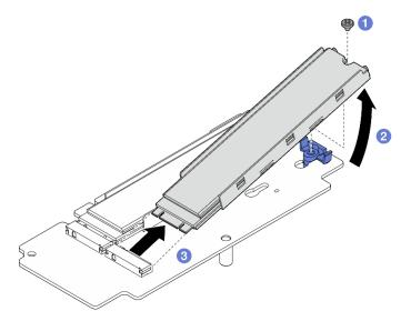
Figure 240. Removing an M.2 drive
