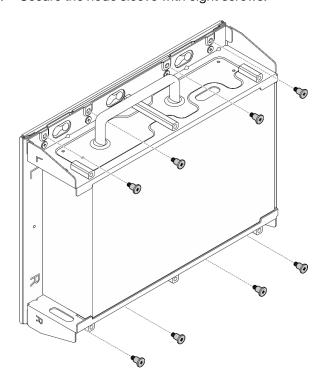
Figure 50. Installing the node bracket
