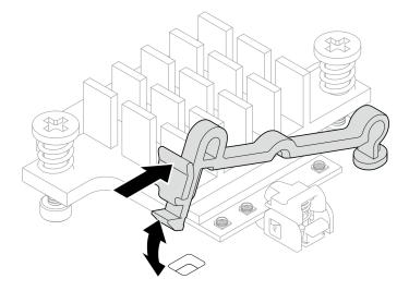
Figure 280. Lifting the cable holder
