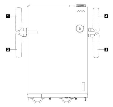
Figure 338. Locations of WLAN antennas
