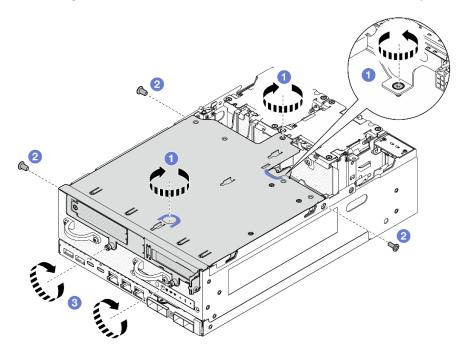
Figure 267. Securing the riser assembly
