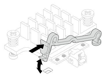
Figure 335. Inserting the cable holder
