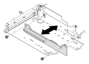
Figure 256. Installing the riser card
