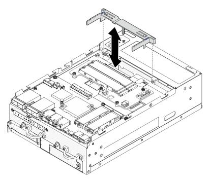
Figure 85. Installing the air baffle
