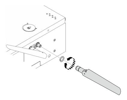
Figure 298. Removing a WLAN antenna
