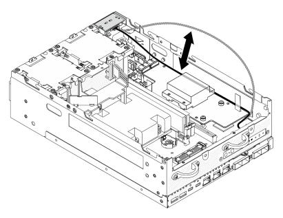
Figure 213. Placing the signal cable
