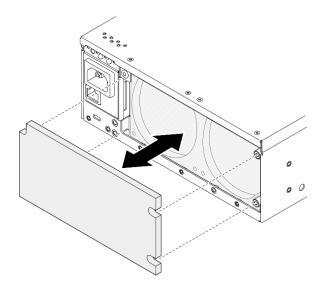
Figure 76. Installing the dust filter
