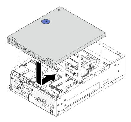
Figure 196. Installing the bottom cover
