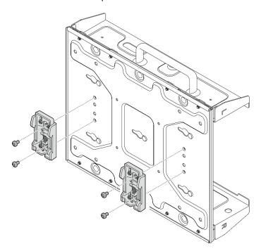
Figure 65. Installing the DIN rail clips
