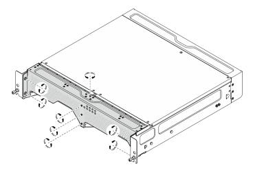
Figure 73. Fastening the screws
