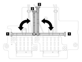
Figure 317. Pivoting the cable holder
