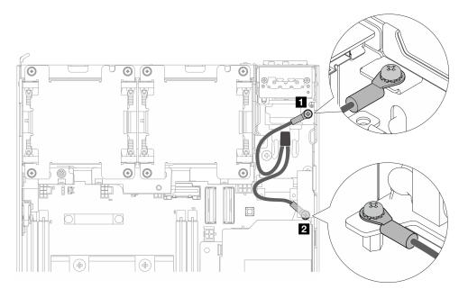
Figure 135. Disconnecting the grounding cables
