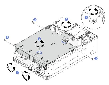
Figure 224. Disengaging the riser assembly
