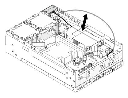
Figure 139. Placing the signal cable
