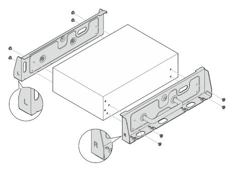
Figure 62. Installing the side brackets with screws
