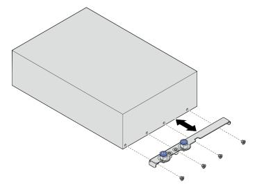
Figure 20. Installing the enclosure bracket
