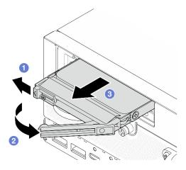
Figure 79. Removing a 7mm drive
