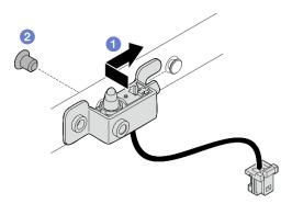
Figure 148. Installing intrusion switch with cable
