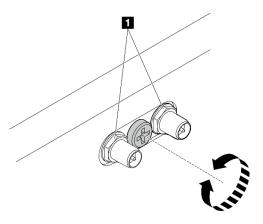
Figure 301. Shortening the SMA connectors
