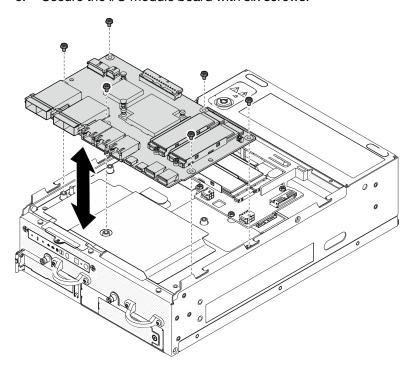
Figure 162. Installing the I/O module board
