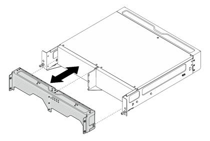
Figure 72. Installing the shipping bracket
