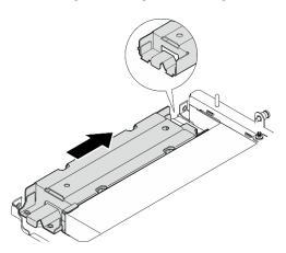
Figure 259. Installing the geotracking module cage
