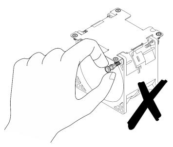
**DO NOT** disassemble the fan module. Attempting to disassemble the fan module might cause damage to the components.
