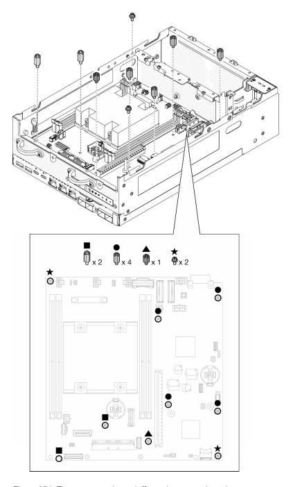
Figure 274. The screws and standoffs on the system board
