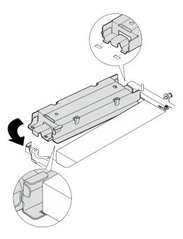
Figure 258. Installing the geotracking module cage
