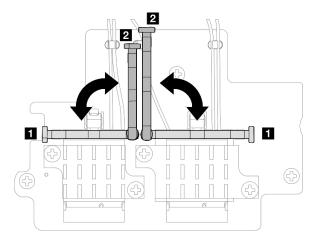
Figure 281. Pivoting the cable holder
