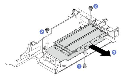
Figure 238. Removing the M.2 adapter
