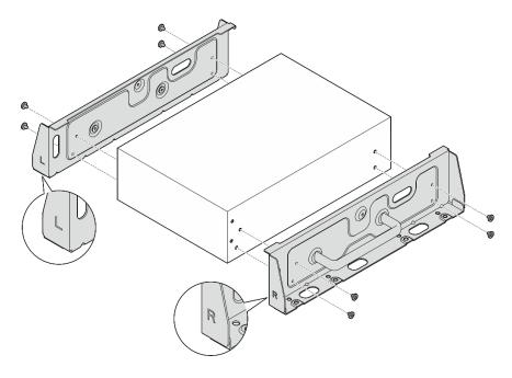
Figure 41. Installing the side brackets with screws
