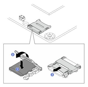
Figure 185. Installing the MicroSD card
