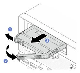
Figure 80. Removing a drive filler
