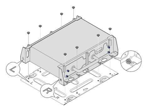
Figure 43. Installing the bottom plate
