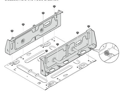
Figure 61. Disassembling the node bracket
