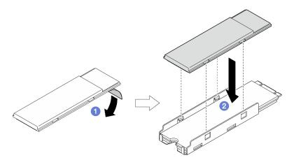
Figure 177. Installing the M.2 heat sink
