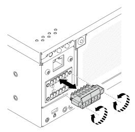
Figure 341. Installing the header
