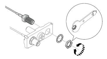
Figure 310. Loosening the cables from the bracket
