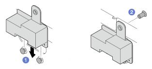
Figure 323. Installing the SMA filler
