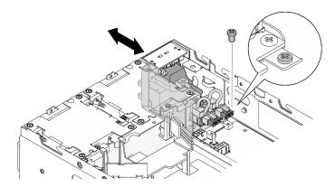
Figure 204. Removing the DC PIB module
