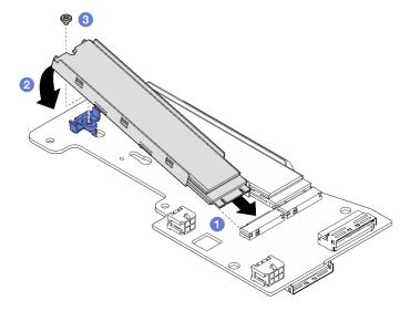
Figure 248. Installing an M.2 drive
