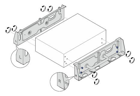
Figure 34. Loosening thumbscrews to remove the side brackets
