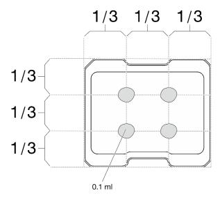
Figure 220. Proper shape of the thermal grease
