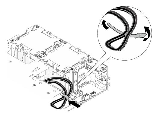
Figure 271. Cable routing for riser assembly
