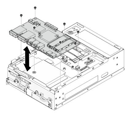
Figure 157. Removing the I/O module board
