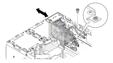
Figure 205. Removing the AC PIB module
