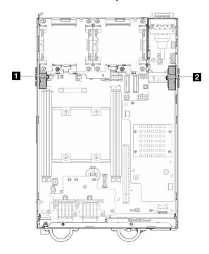
Figure 325. SMA assembly locations
