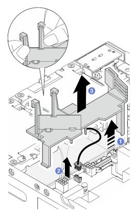
Figure 89. Removing the air baffle
