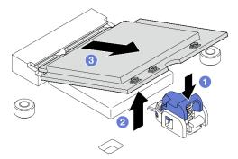
Figure 284. Removing the WLAN/Bluetooth module
