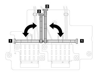
Figure 110. Pivoting the cable holder
