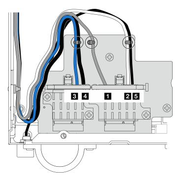
Figure 332. Cable routing for wireless adapter
