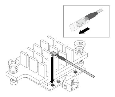
Figure 293. Connecting the cable
