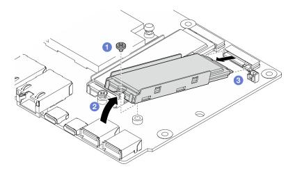
Figure 156. Removing an M.2 drive
