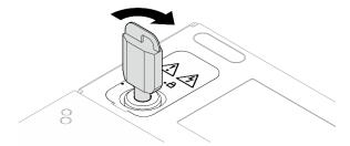
Figure 188. Locking the keylock
