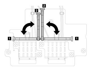
Figure 294. Pivoting the cable holder
