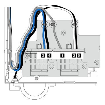
Figure 292. Cable routing for wireless adapter
