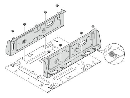
Figure 59. Assembling the node sleeve
