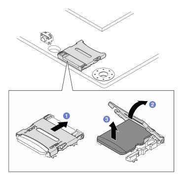
Figure 184. Removing the MicroSD card
