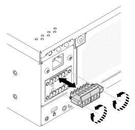
Figure 207. Removing the header
