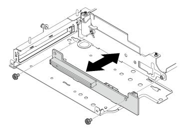
Figure 237. Removing the riser card
