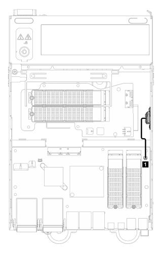
Figure 155. Bottom intrusion switch cable routing
