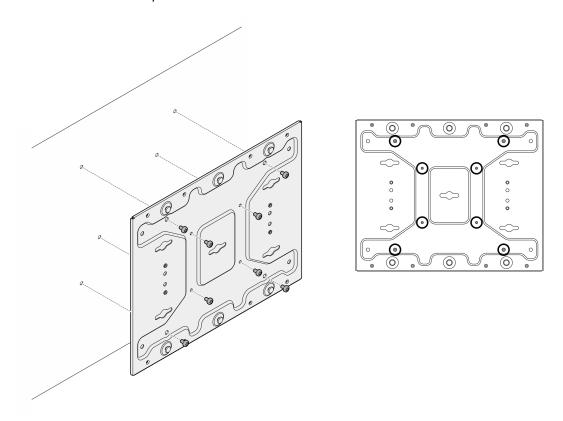
Figure 46. Installing the wall-mount plate
