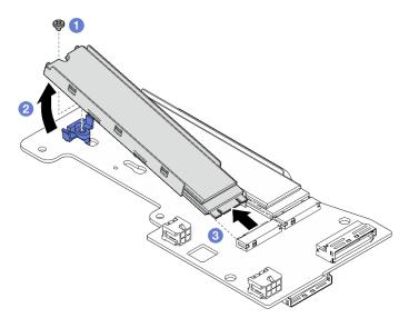
Figure 114. Removing an M.2 drive
