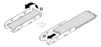
Figure 176. Installing the M.2 drive
