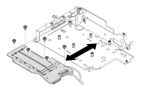
Figure 227. Removing the M.2 cabled adapter
