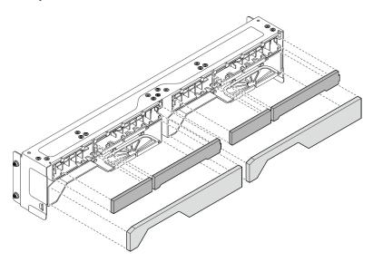
Figure 71. Installing the dust filters
