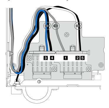
Figure 345. WLAN antenna and Bluetooth antenna cable routing
