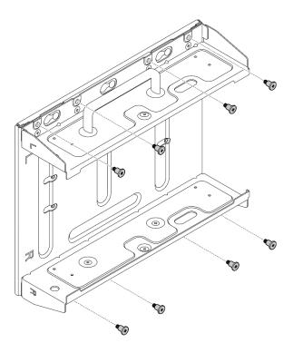
Figure 27. Removing the node bracket
