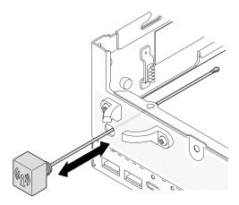
Figure 102. Removing the Bluetooth antenna
