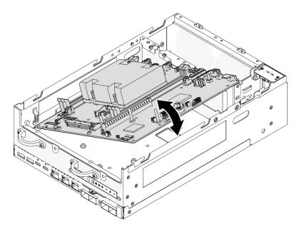
Figure 275. Removing the system board
