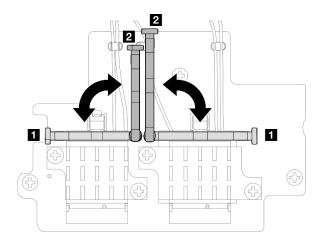
Figure 108. Pivoting the cable holder
