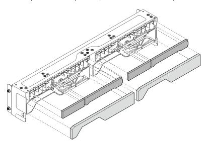
Figure 70. Removing the dust filters
