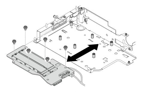
Figure 250. Installing the M.2 adapter
