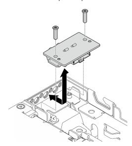
Figure 223. Installing the rear operator panel
