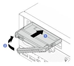
Figure 82. Installing a drive filler
