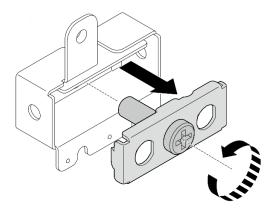
Figure 326. Removing the bracket
