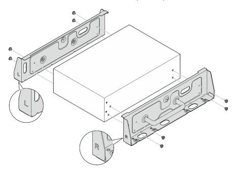
Figure 33. Loosening screws to remove the side brackets
