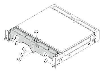
Figure 68. Loosening the screws
