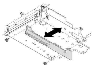
Figure 252. Installing the riser card
