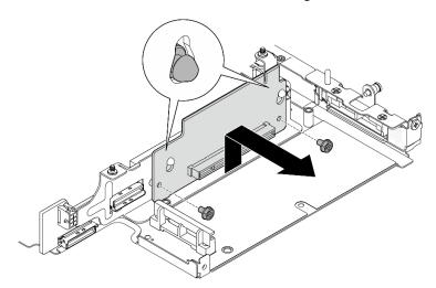
Figure 239. Removing the riser card
