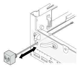
Figure 105. Installing the Bluetooth antenna
