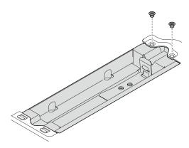
Figure 234. Removing the geotracking module cage
