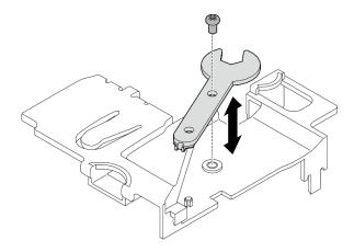
Figure 324. Disengaging the wrench
