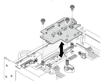
Figure 286. Installing the wireless adapter
