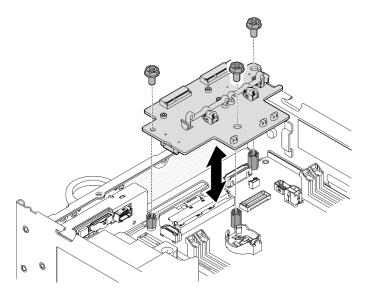
Figure 285. Removing the wireless adapter
