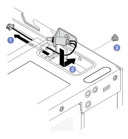
Figure 171. Installing the lock position switch with cable
