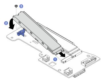
Figure 118. Installing an M.2 drive
