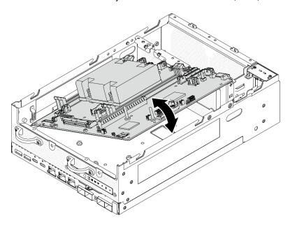
Figure 276. Installing the system board
