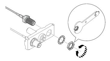
Figure 327. Fastening the cables to the bracket
