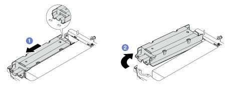
Figure 235. Removing the geotracking module cage
