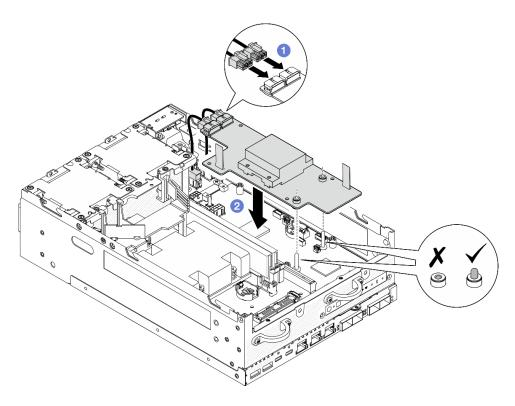
Figure 214. Installing the power module board
