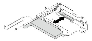
Figure 236. Removing the PCIe adapter
