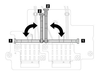
Figure 334. Pivoting the cable holder
