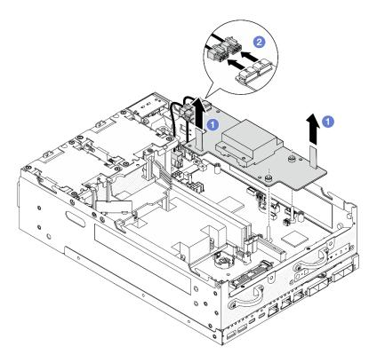
Figure 212. Removing the power module board
