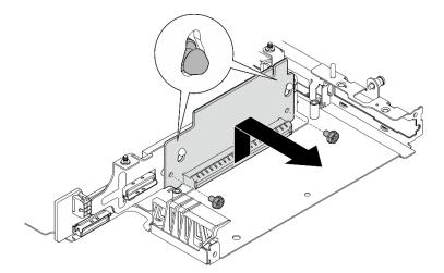
Figure 242. Removing the riser card
