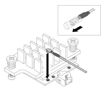
Figure 109. Connecting the cable
