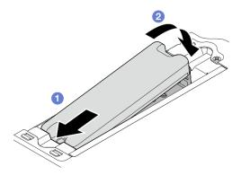
Figure 261. Installing the geotracking module
