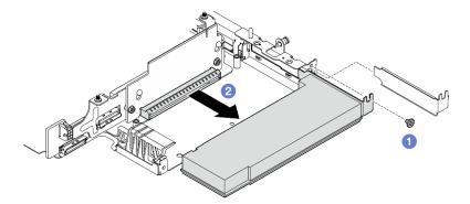
Figure 241. Removing the PCIe adapter
