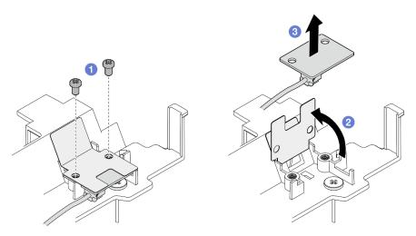
Figure 90. Removing the air flow sensor board
