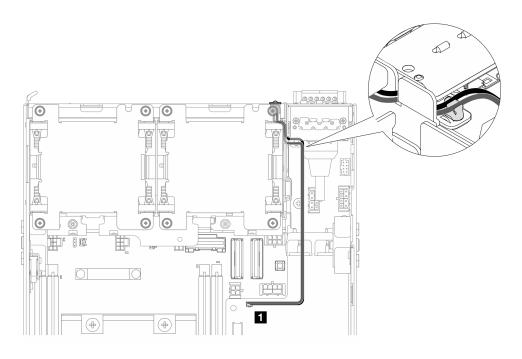
Figure 198. PMB status LED cable connecting to the DC power module board (DC PMB)
