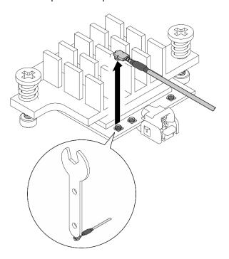
Figure 282. Disconnecting the cable
