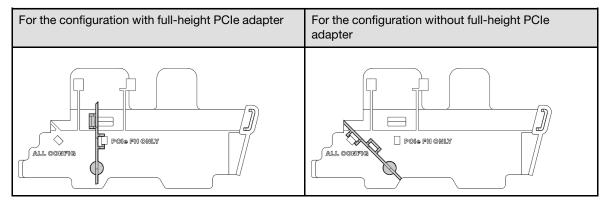
Step 3. Align the front of the riser assembly with the edge of the chassis; then, lower the riser assembly to the node.
