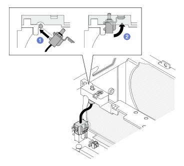
Figure 126. Installing intrusion switch with cable
