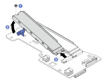
Figure 228. Removing an M.2 drive
