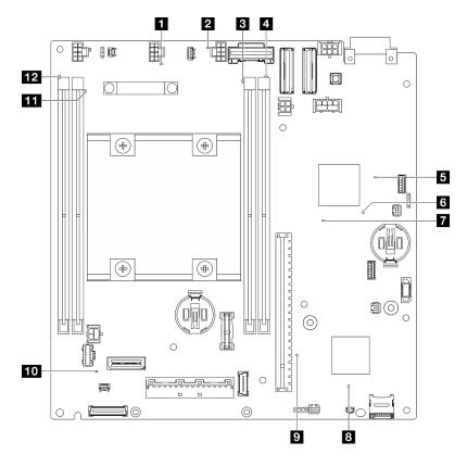
Figure 353. System-board LEDs
