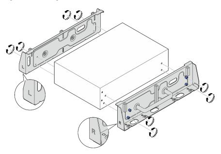
Figure 58. Loosening thumbscrews to remove the side brackets
