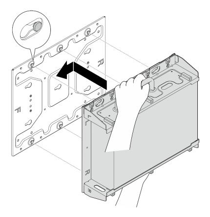
Figure 49. Installing the node bracket
