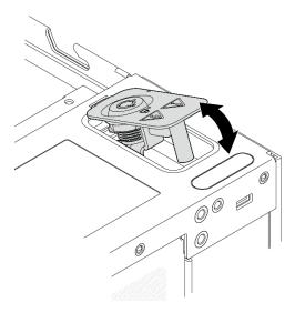
Figure 173. Installing the system security keylock
