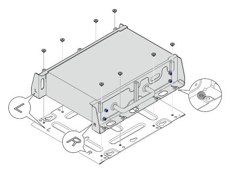
Figure 32. Removing the bottom plate
