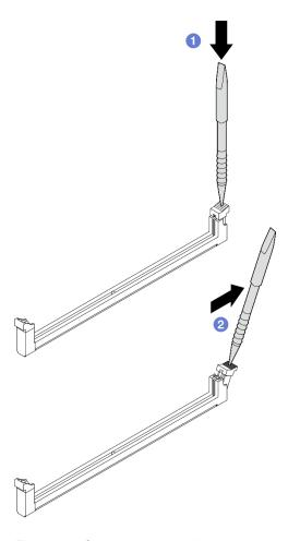
Figure 179. Opening retaining clip
