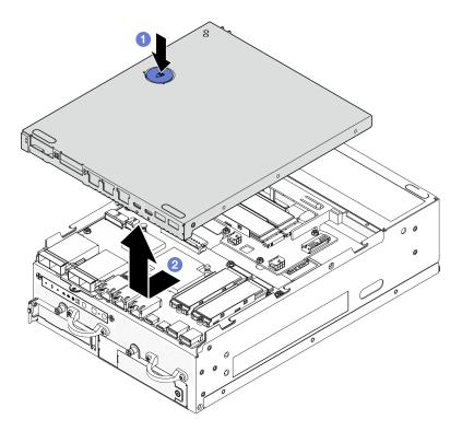
Figure 193. Removing bottom cover
