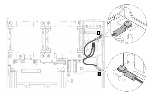
Figure 142. Connecting the grounding cable
