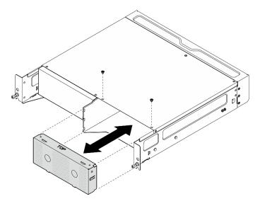
Figure 5. Installing the node filler
