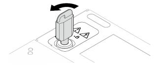
Figure 195. Unlocking the keylock
