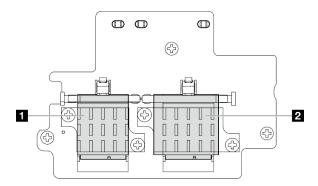
x86 WLAN module (with two cable connectors)
