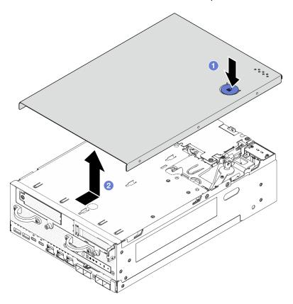
Figure 187. Removing the top cover
