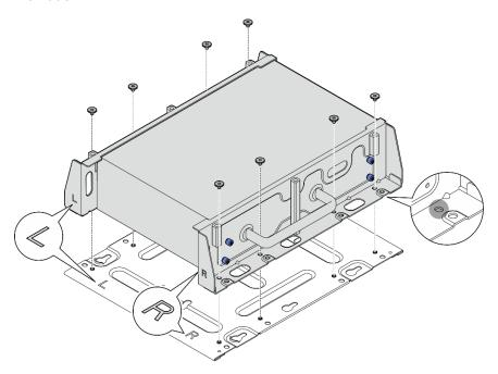
Figure 56. Removing the bottom plate
