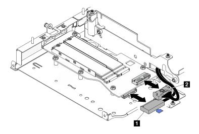
Figure 251. Disconnecting the signal cable
