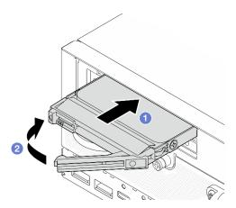
Figure 81. Installing a 7mm drive
