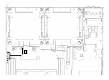
Figure 144. Top intrusion switch cable routing
