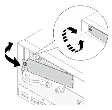
Figure 78. Removing the bezel
