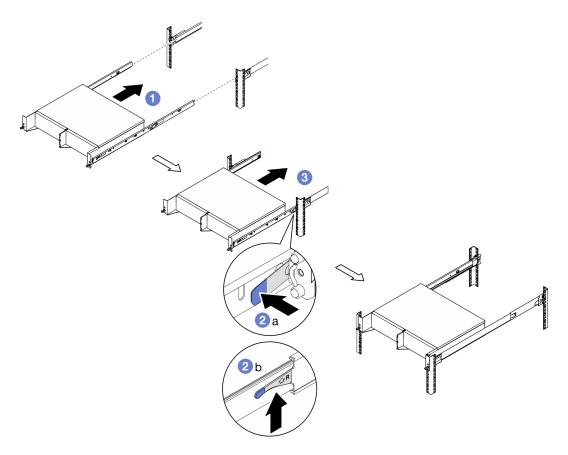
Figure 17. Installing the enclosure to the rack
