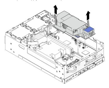
Figure 138. Removing the internal power supply unit
