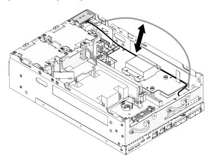
Figure 209. Placing the signal cable
