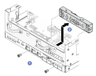
Figure 132. Removing the front operator panel
