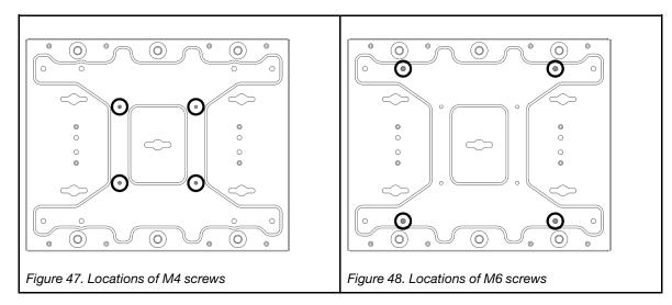
Step 12. Install the node bracket to the wall-mount plate.
