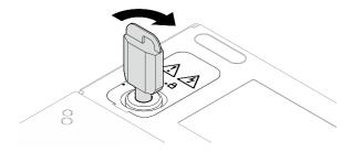
Figure 197. Locking the keylock
