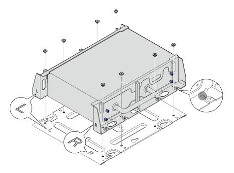
Figure 64. Installing the bottom plate
