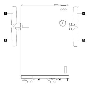
Figure 297. Locations of WLAN antennas
