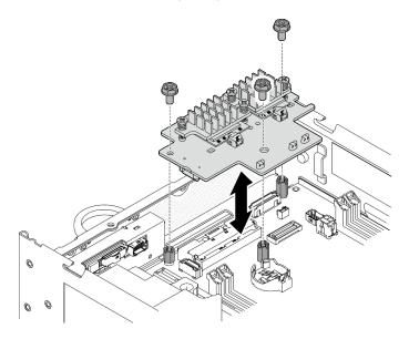
Figure 95. Lifting the wireless adapter
