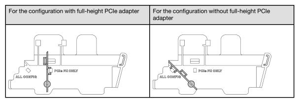
Step 3. Align the front of the riser assembly with the edge of the chassis; then, lower the riser assembly to the node.
