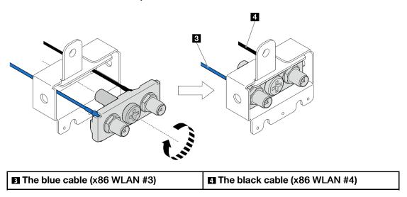
Step 6. Install the SMA assembly.
