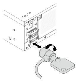
Figure 165. Removing the Kensington lock
