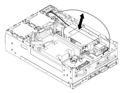
Figure 134. Placing the signal cable
