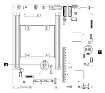
Figure 119. CMOS battery locations on the system board
