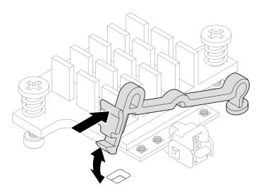
Figure 100. Inserting the cable holder
