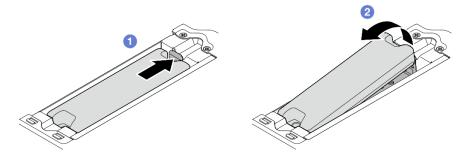
Figure 233. Removing the geotracking module
