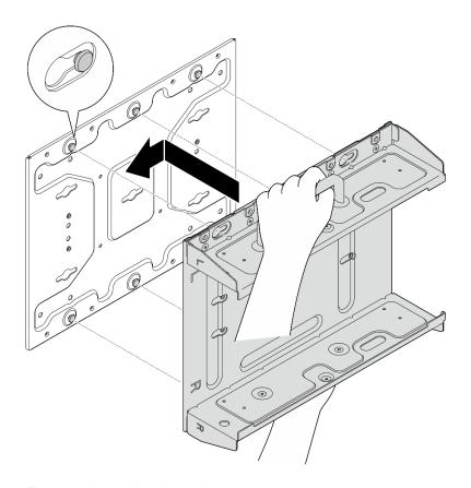
Figure 36. Assembling the node sleeve
