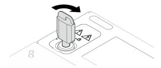
Figure 191. Locking the keylock
