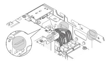
Figure 215. The slots for PMB air baffle
