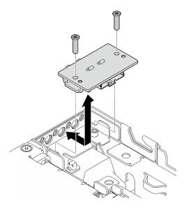
Figure 222. Removing the rear operator panel
