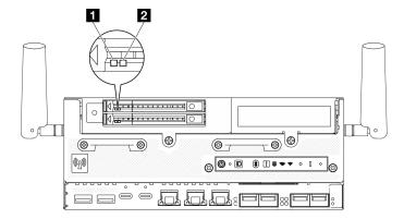
Figure 349. Drive LEDs
