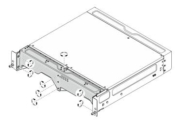
Figure 25. Fastening the screws
