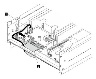
Figure 159. I/O-board cable routing
