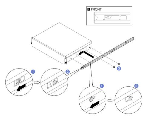
Figure 16. Installing the inner rail
