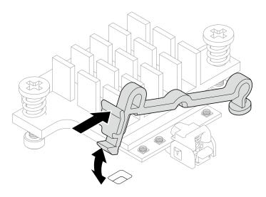
Figure 96. Lifting the cable holder
