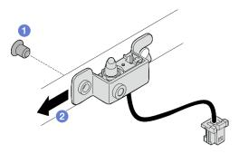
Figure 145. Removing intrusion switch with cable
