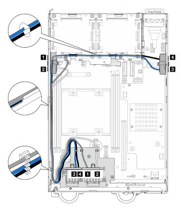
Figure 329. Cable routing for the SMA assemblies
