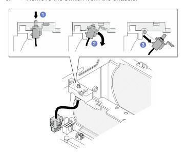
Figure 125. Removing the fan direction switch
