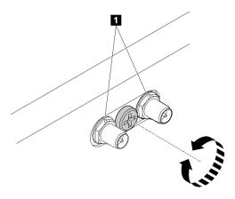
Figure 54. Shortening the SMA connectors
