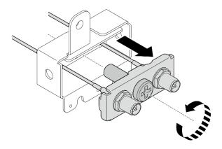
Figure 309. Removing the bracket
