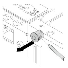
Figure 200. Removing the PMB status LED cable
