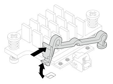
Figure 295. Inserting the cable holder
