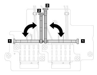
Figure 304. Pivoting the cable holder
