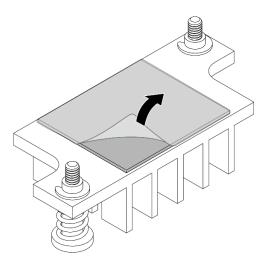
Figure 290. Removing the film from thermal pad
