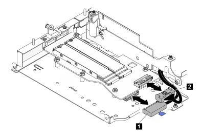
Figure 226. Disconnecting the signal cable
