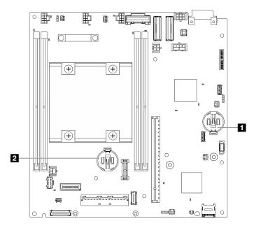
Figure 122. CMOS battery locations on the system board
