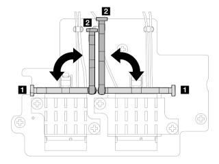
Figure 315. Pivoting the cable holder
