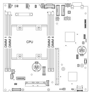
Figure 1. Memory modules and processor layout
