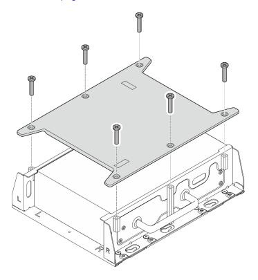
Figure 44. Installing the reinforced cover
