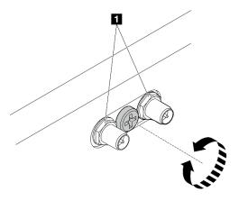
Figure 40. Shortening the SMA connectors
