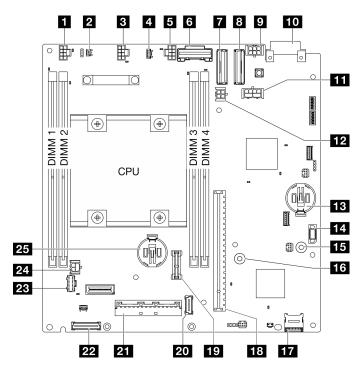
Figure 348. System-board connectors
