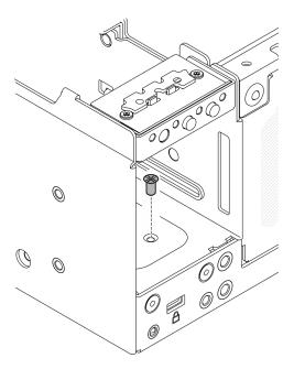
Figure 167. Loosening the screw
