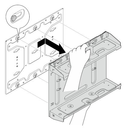
Figure 28. Removing the node bracket
