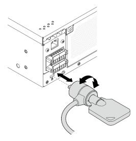
Figure 166. Installing the Kensington lock
