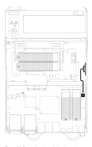
Figure 150. Bottom intrusion switch cable routing
