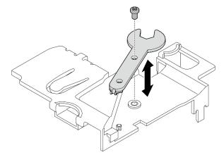
Figure 300. Disengaging the wrench
