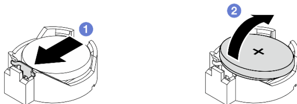
Figure 118. Removing the CMOS battery
