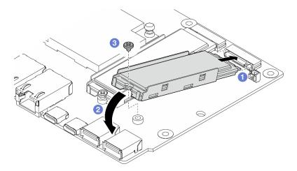
Figure 164. Installing an M.2 drive
