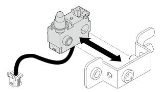
Figure 146. Separating the intrusion switch from the bracket
