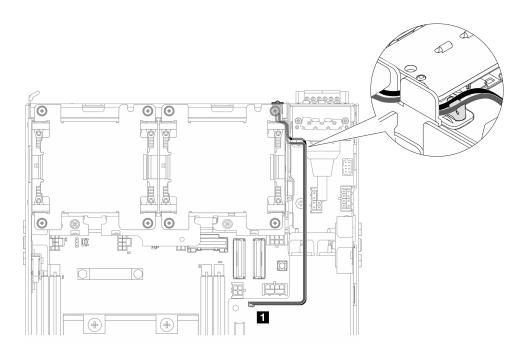
Figure 202. PMB status LED cable connecting to the DC power module board (DC PMB)
