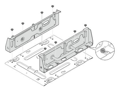
Figure 39. Disassembling the node bracket
