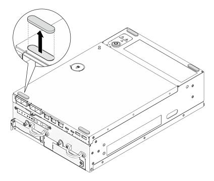
Figure 272. Removing the rubber feet
