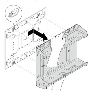
Figure 38. Separating the node bracket
