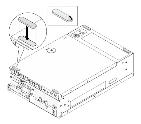
Figure 273. Installing the rubber feet
