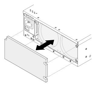
Figure 75. Removing the dust filter
