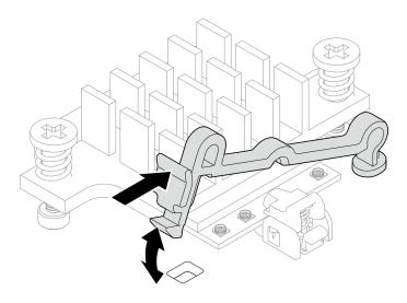
Figure 307. Inserting the cable holder
