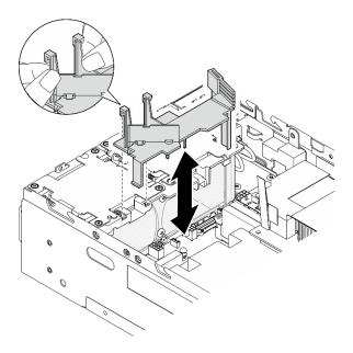
Figure 88. Removing the air baffle
