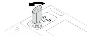
Figure 186. Unlocking the keylock
