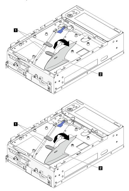
Figure 161. I/O-board cable routing
