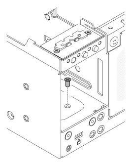
Figure 174. Fastening the screw
