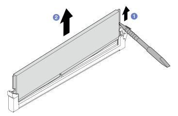
Figure 180. Removing memory module
