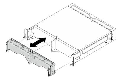
Figure 3. Removing the shipping bracket
