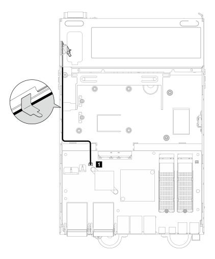
Figure 169. Lock position switch cable routing
