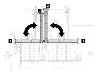
Figure 97. Pivoting the cable holder
