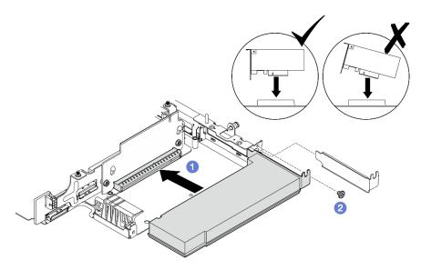
Figure 247. Installing the PCIe adapter
