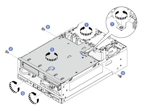
Figure 263. Securing the riser assembly
