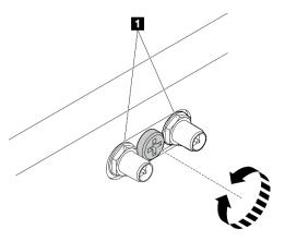
Figure 31. Shortening the SMA connectors
