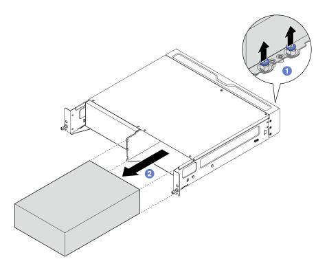
Figure 4. Removing the node
