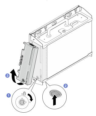
Figure 52. Removing the security bezel
