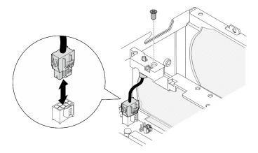
Figure 127. Installing the fan direction switch
