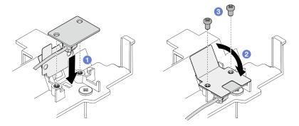
Figure 92. Installing the air flow sensor board
