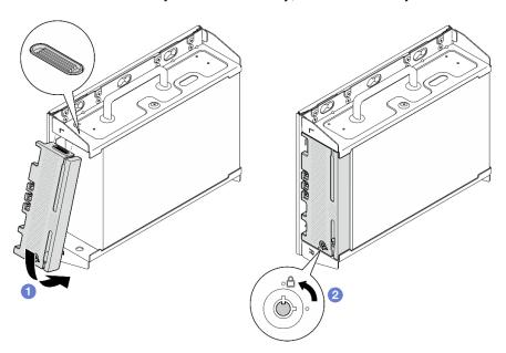
Figure 67. Installing the security bezel
