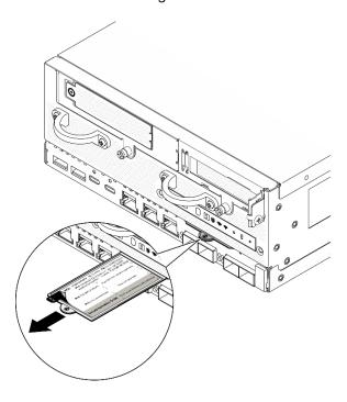
Figure 279. Lenovo XClarity Controller network access label on the pull-out information tab
