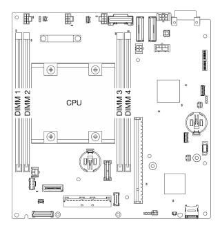
Figure 181. Memory modules and processor layout
