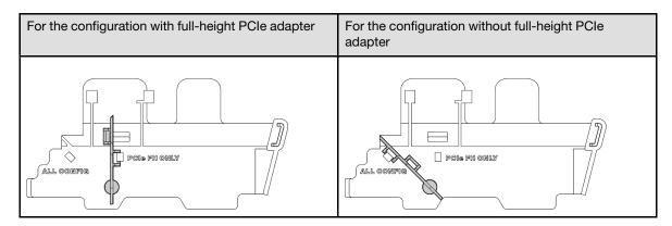
Step 4. Align the front of the riser assembly with the edge of the chassis; then, lower the riser assembly to the node.
