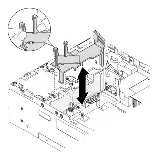
Figure 91. Installing the air baffle
