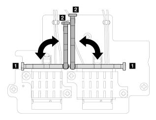
Figure 99. Pivoting the cable holder
