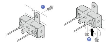
Figure 308. Removing the SMA assembly
