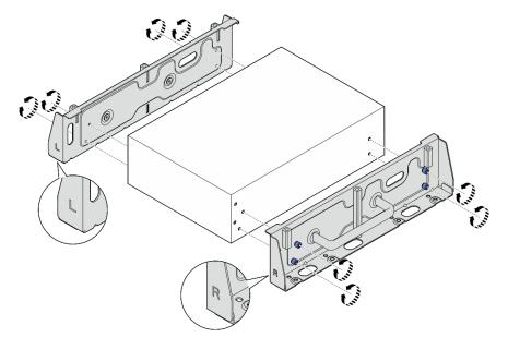
Figure 42. Installing the side brackets with thumbscrews
