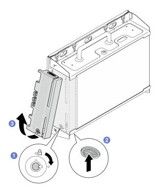
Figure 26. Removing the security bezel
