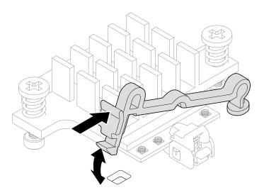
Figure 107. Lifting the cable holder
