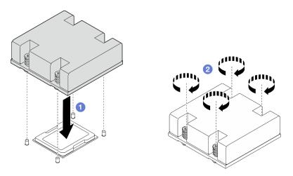
Figure 221. Installing the processor heat sink
