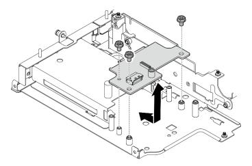
Figure 254. Installing Backplane 1
