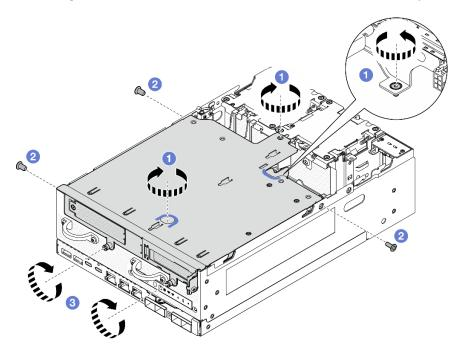
Figure 270. Securing the riser assembly
