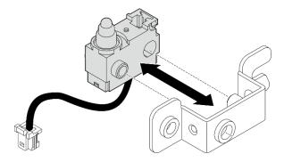
Figure 147. Inserting the intrusion switch to the bracket
