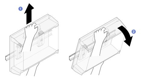
Figure 53. Removing the node sleeve
