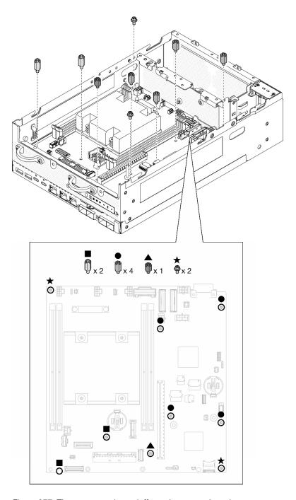
Figure 277. The screws and standoffs on the system board
