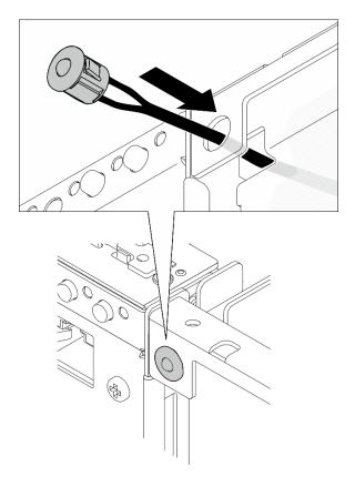
Figure 201. Installing the PMB status LED cable
