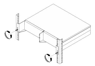
Figure 18. Securing the enclosure to the rack
