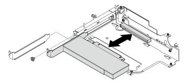
Figure 257. Installing the PCIe adapter
