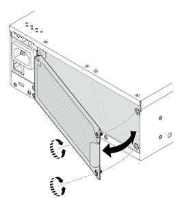
Figure 74. Removing the bezel
