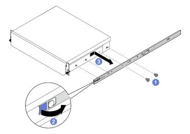
Figure 9. Removing the inner rail
