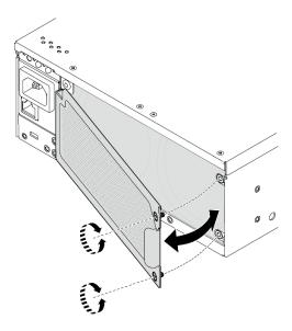
Figure 77. Installing the bezel
