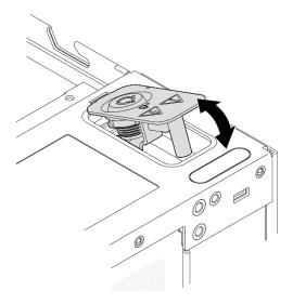
Figure 168. Removing the system security keylock
