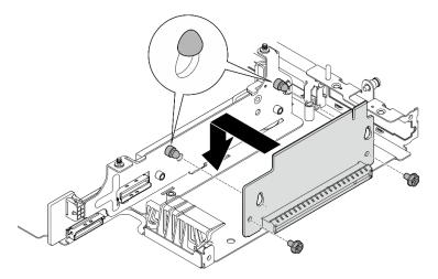
Figure 246. Installing the riser card
