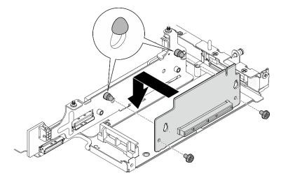
Figure 244. Installing the riser card
