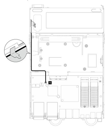
Figure 172. Lock position switch cable routing
