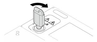
Figure 194. Locking the keylock
