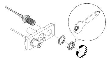
Figure 321. Loosening the cables from the bracket
