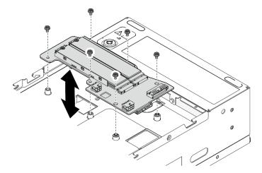
Figure 117. Installing the bottom M.2 cabled adapter
