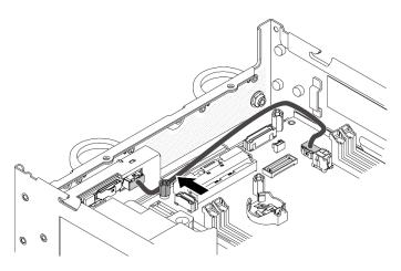
Figure 343. Front operator panel cable routing
