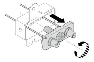
Figure 320. Removing the bracket
