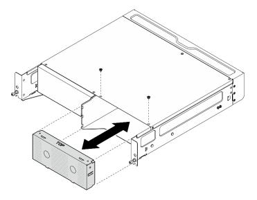
Figure 23. Installing the node filler
