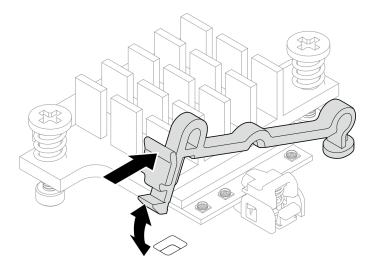
Figure 303. Lifting the cable holder
