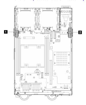
Figure 299. SMA assembly locations
