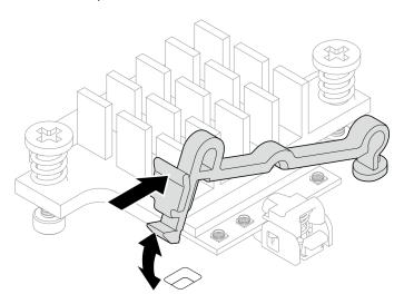
Figure 314. Lifting the cable holder
