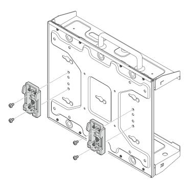
Figure 55. Removing the DIN rail clips
