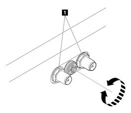
Figure 312. Shortening the SMA connectors
