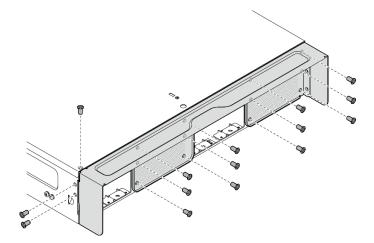
Figure 10. Loosening the screws
