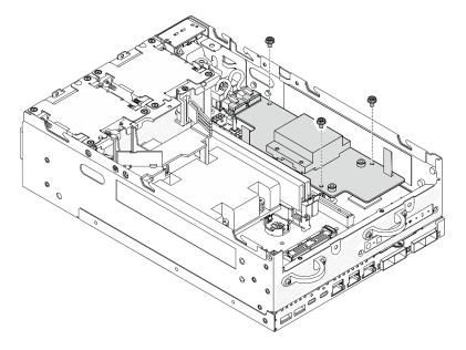
Figure 211. Loosening the screws
