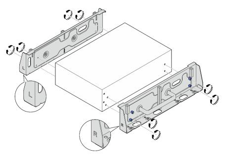
Figure 63. Installing the side brackets with thumbscrews
