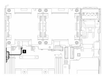
Figure 149. Top intrusion switch cable routing
