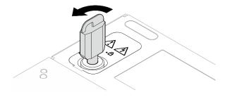
Figure 192. Unlocking the keylock
