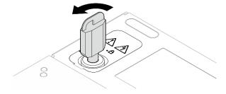
Figure 189. Unlocking the keylock
