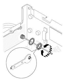
Figure 101. Removing the Bluetooth antenna
