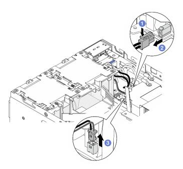
Figure 136. Disconnecting the cables
