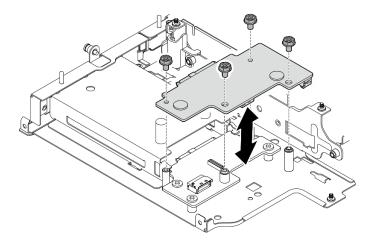
Figure 255. Installing Backplane 2
