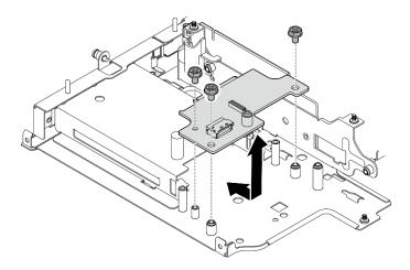
Figure 232. Removing Backplane 1
