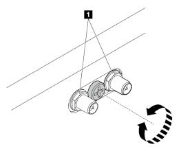
Figure 60. Shortening the SMA connectors
