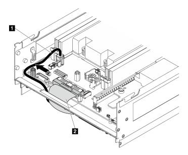
Figure 278. I/O-board cable routing
