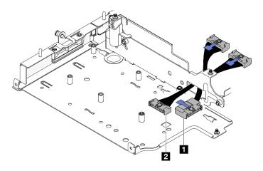
Figure 249. M.2 cabled adapter signal cable
