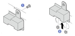
Figure 313. Removing the SMA filler
