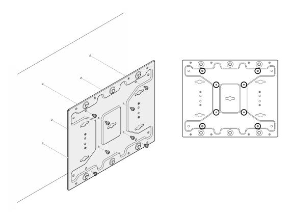
Figure 29. Removing the wall-mount plate
