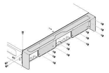
Figure 13. Fastening the screws
