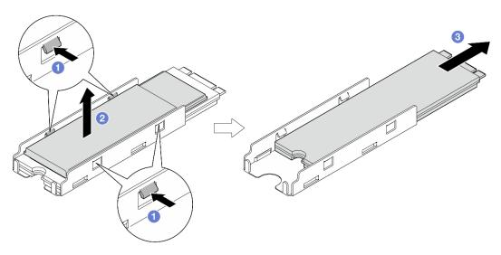
Figure 175. Removing the M.2 heat sink
