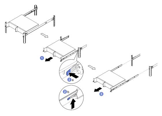
Figure 8. Removing the enclosure from the rack
