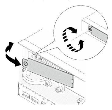
Figure 83. Installing the bezel
