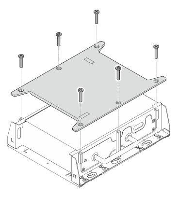
Figure 30. Removing the reinforced cover
