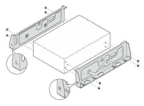
Figure 57. Loosening screws to remove the side brackets
