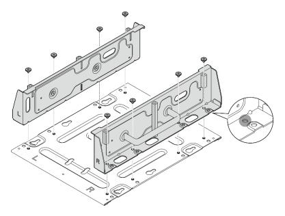
Figure 35. Assembling the node sleeve
