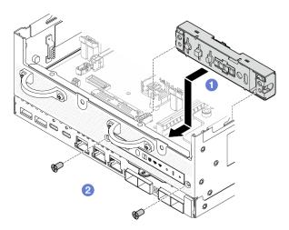
Figure 133. Installing the front operator panel
