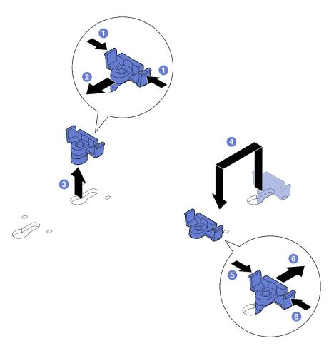
Figure 116. Adjusting the M.2 retainer
