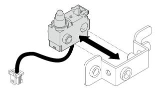
Figure 152. Separating the intrusion switch from the bracket
