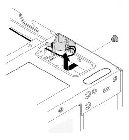
Figure 170. Removing the lock position switch with cable
