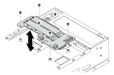
Figure 115. Removing the bottom M.2 cabled adapter
