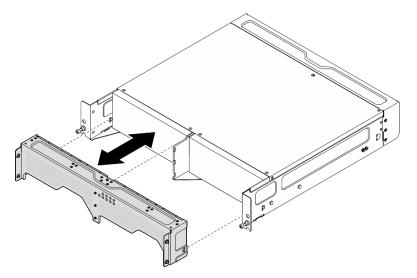
Figure 24. Installing the shipping bracket
