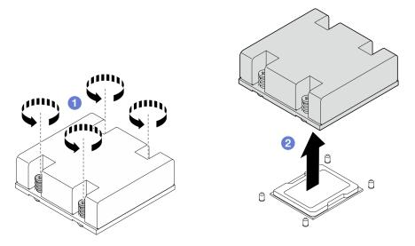
Figure 219. Removing the processor heat sink
