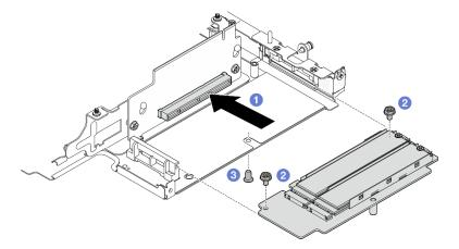
Figure 245. Installing the M.2 adapter
