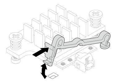
Figure 330. Lifting the cable holder
