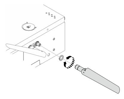
Figure 340. Installing a WLAN antenna
