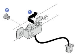
Figure 154. Installing intrusion switch with cable
