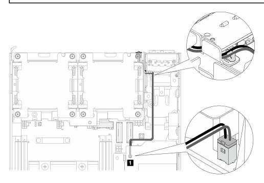
Figure 199. PMB status LED cable connecting to the internal power supply unit (AC PMB)
