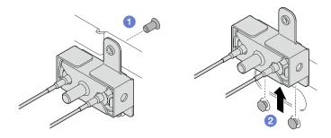
Figure 319. Removing the SMA assembly
