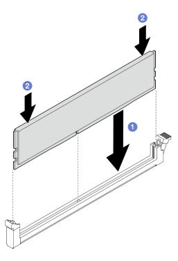
Figure 183. Installing a memory module
