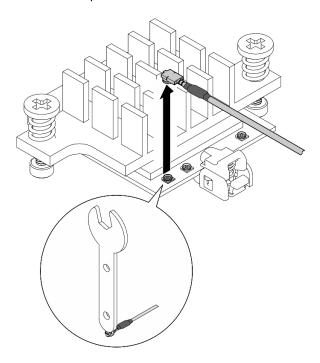
Figure 316. Disconnecting the cable
