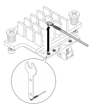
Figure 305. Disconnecting the cable
