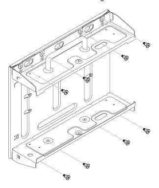
Figure 37. Assembling the node sleeve
