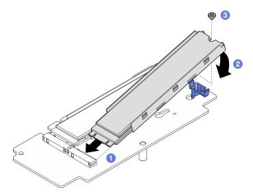
Figure 243. Installing an M.2 drive
