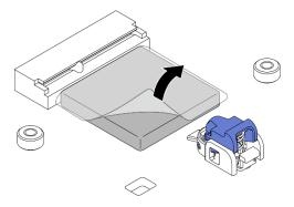
Figure 288. Removing the film from thermal pad
