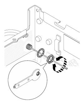
Figure 106. Installing the Bluetooth antenna
