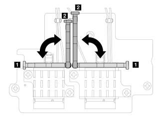
Figure 331. Pivoting the cable holder
