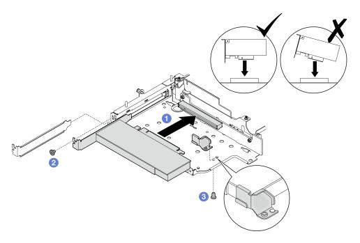
Figure 253. Installing the PCIe adapter
