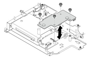
Figure 231. Removing Backplane 2
