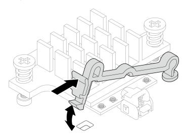
Figure 318. Inserting the cable holder
