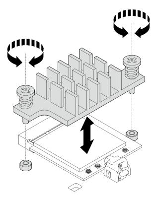
Figure 283. Removing the WLAN/Bluetooth module heat sink
