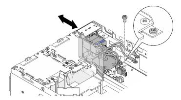
Figure 208. Installing the PIB module
