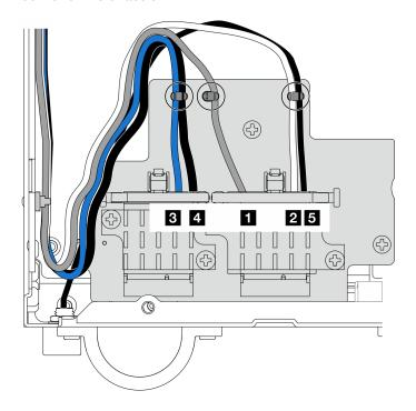
Figure 336. Cable routing for wireless adapter
