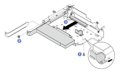
Figure 229. Removing the PCle adapter
