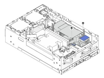
Figure 137. Loosening the screws
