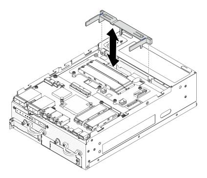
Figure 84. Removing the air baffle
