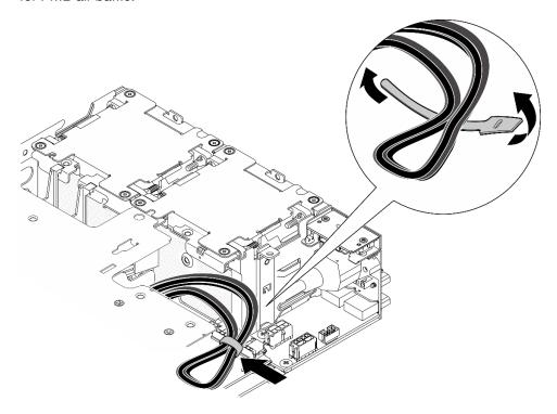
Figure 264. Cable routing for riser assembly
