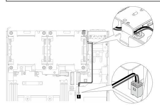
Figure 203. PMB status LED cable connecting to the internal power supply unit (AC PMB)
