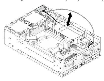
Figure 143. Placing the signal cable
