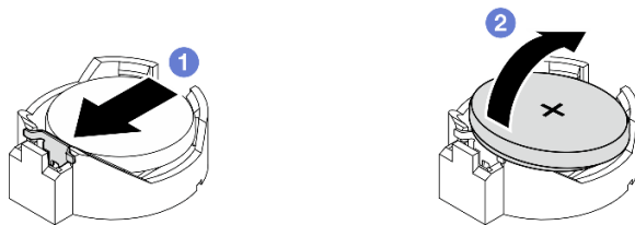
Figure 138. Removing the CMOS battery
