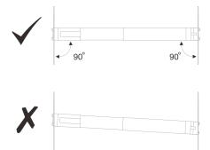
Step 2. Open the front mounting bracket, and align the front pins of the outer rail to the holes in the rack. Pull the outer rail as shown until the pins are inserted into the corresponding holes.
