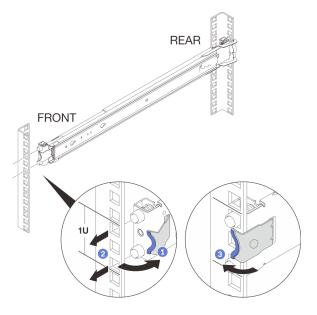
Repeat the previous steps to install the rear and front mounting bracket of the other rail.
