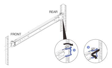
Repeat the previous steps to remove the front and rear mounting bracket of the other rail.
