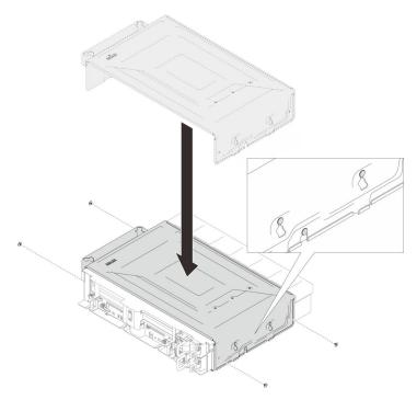
Step 3. Hold the top handle, and lower the assembly into the floor stand. Then, secure each side of the assembly to the server stand with two **large** M3 screws.
