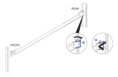
Repeat the previous steps to remove the front and rear mounting bracket of the other rail.
