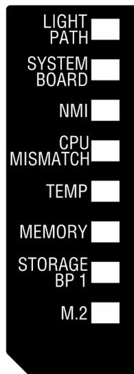
Figura 6. LED del pannello LPD (Lightpath Diagnostics)
