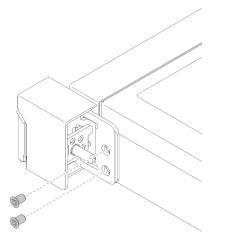
Figure 66. Rack latches removal
