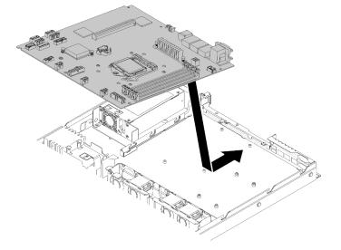
Figure 77. System board installation
