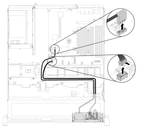
Figure 41. Front operator panel removal
