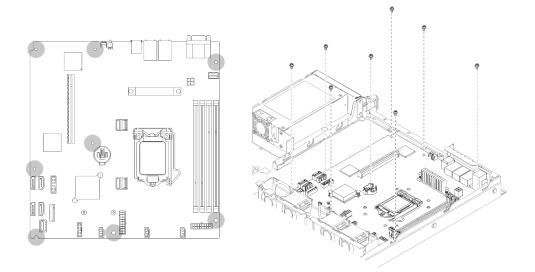
Figure 78. System-board screws location
