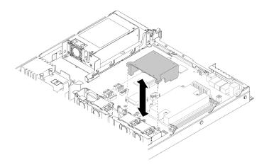
Figure 25. Air baffle removal
