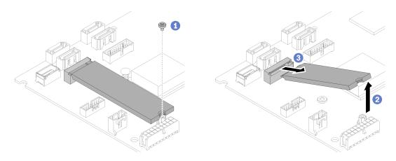
Figure 50. M.2 drive removal
