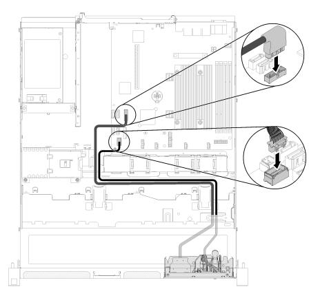
Figure 46. Front operator panel installation
