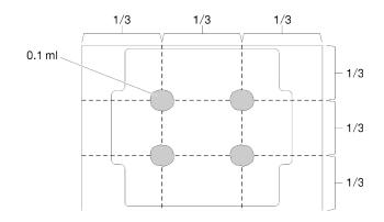
Figure 62. Proper shape of the thermal grease
