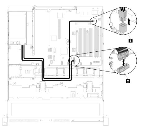
Figure 18. Fixed power supply unit cables
