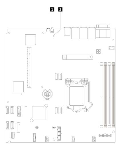
Figure 93. System-board LEDs
