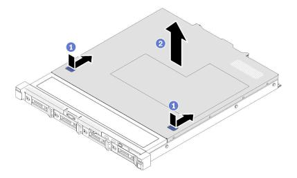
Figure 79. Top cover removal
