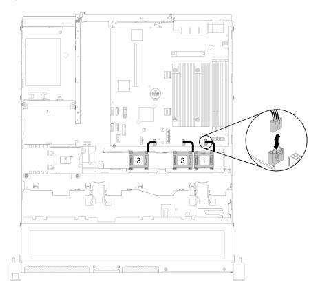
Figure 16. Fan cables
