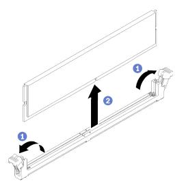
Figure 30. DIMM removal
