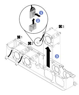
Figure 37. Fan removal
