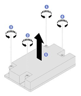
Figure 47. Heat sink removal
