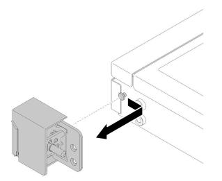
Figure 67. Rack latches removal
