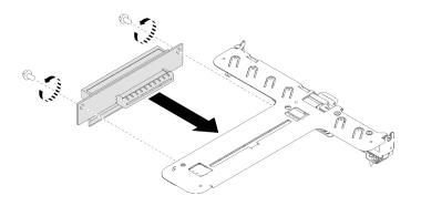
Figure 56. PCIe riser assembly installation
