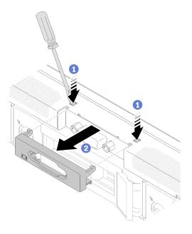
Figure 84. VGA cable removal
