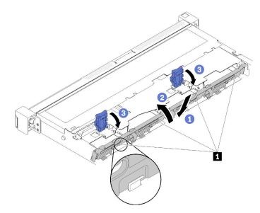
Figure 36. Simple-swap drive backplate installation
