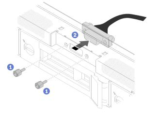
Figure 85. VGA cable removal
