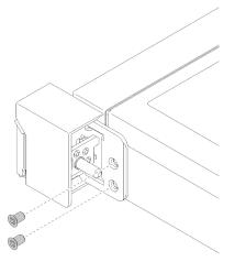
Figure 69. Rack latches installation
