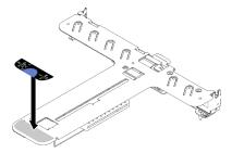
Figure 57. PCIe riser assembly installation
