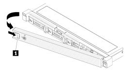
Figure 72. Security bezel removal
