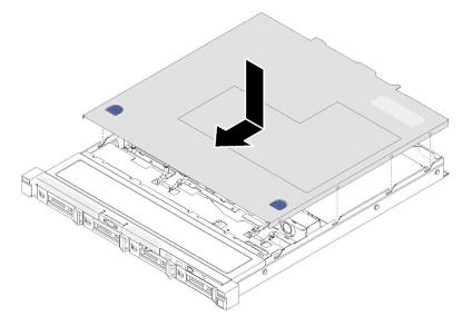
Figure 80. Top cover installation
