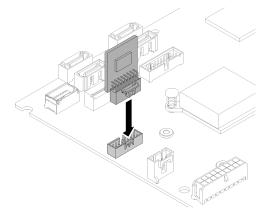
Figure 82. TPM card installation
