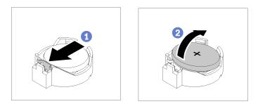
Figure 27. CMOS battery removal
