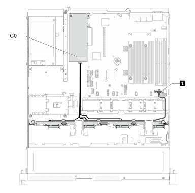
Figure 21. 3.5-inch simple-swap drive model with hardware RAID
