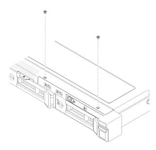
Figure 42. Front operator panel removal
