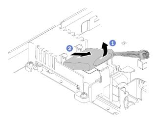
Figure 39. Flash power module removal
