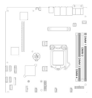
Figure 29. DIMM connectors
