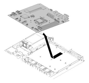
Figure 76. System board removal
