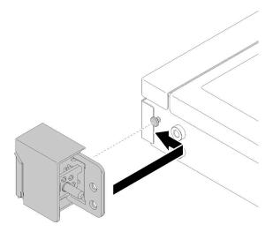
Figure 68. Rack latches installation
