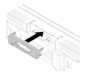
Figure 88. VGA cable installation
