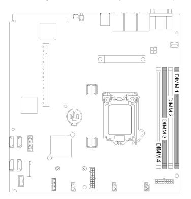
Figure 31. DIMM connectors
