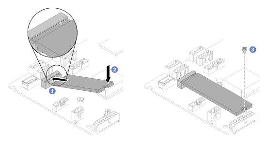
Figure 53. M.2 drive installation
