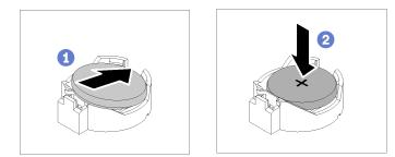
Figure 28. CMOS battery installation
