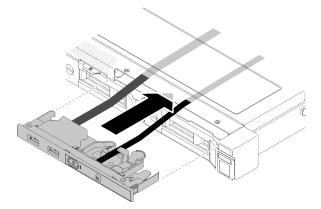
Figure 44. Front operator panel installation
