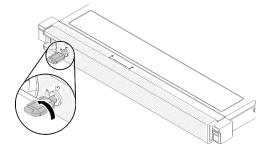
Figure 74. Locking the security bezel
