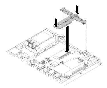
Figure 58. PCIe riser assembly installation
