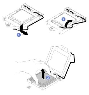
Figure 61. Opening the processor retainer
