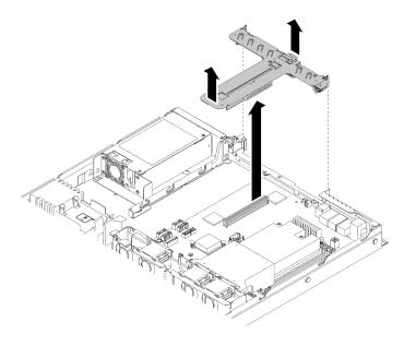
Figure 54. PCIe riser assembly removal
