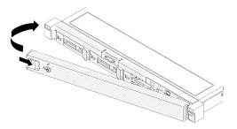
Figure 73. Security bezel installation
