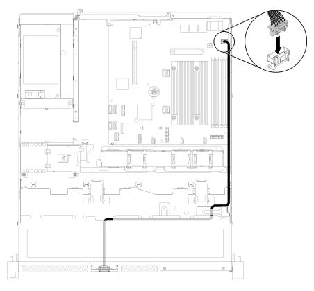
Figure 87. VGA cable installation
