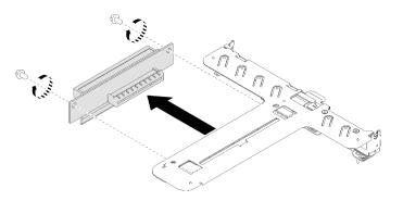
Figure 55. PCIe riser assembly removal
