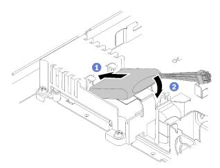
Figure 40. Flash power module installation
