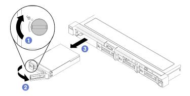
Figure 33. Simple-swap disk drive removal
