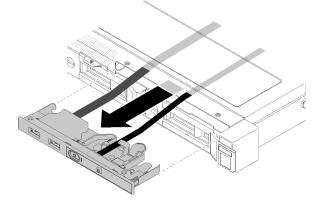
Figure 43. Front operator panel removal
