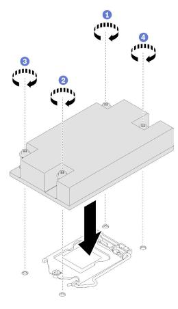
Figure 48. Heat sink installation
