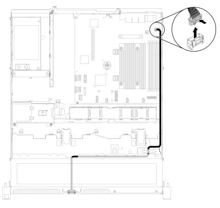
Figure 83. VGA cable removal
