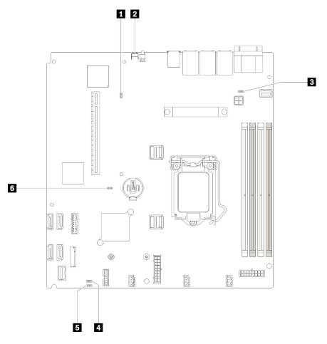
Figure 10. System-board jumpers and buttons
