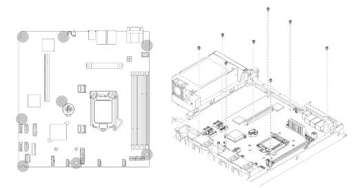
Figure 75. System-board screws location
