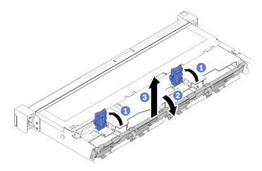
Figure 35. Simple-swap drive backplate removal
