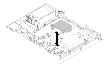
Figure 26. Air baffle installation
