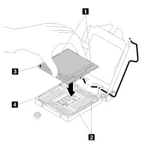
Figure 63. Installing the processor
