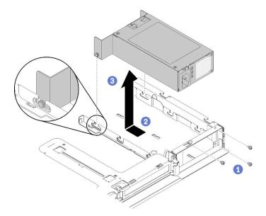
Figure 59. Power supply unit removal
