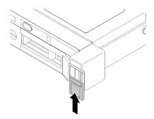
Figure 70. ID label installation
