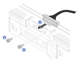
Figure 86. VGA cable installation
