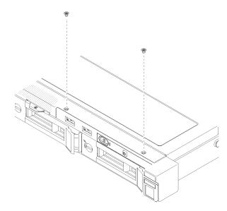
Figure 45. Front operator panel installation
