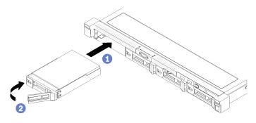
Figure 34. Simple-swap disk drive installation
