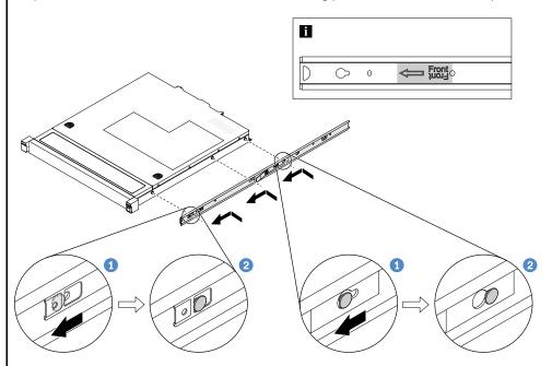
**Note**1: Make sure the stamp "Front" always face toward the front when assemble the inner rail to the server or to the slide-rail assembly.
