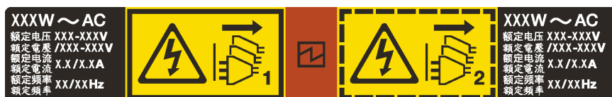
Figure 63. Hot-swap power supply label on the cover
