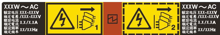
Figure 38. Hot-swap power supply label on the cover
