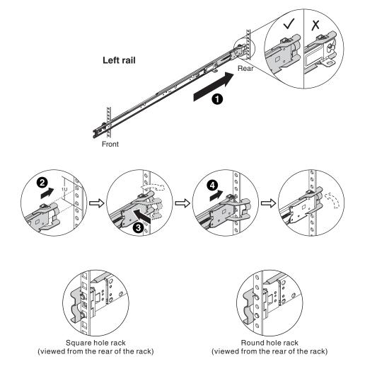
2. Install the front mounting bracket of the left rail.
