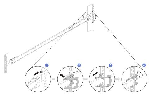
**Note:** When install the rail to the vertical rack, use left rail as top rail, and right rail as bottom rail. Installation methods are the same in both racks.
