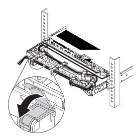
7. Use the cable straps provided to secure the cables. Cables must be bundled with cable straps for proper movement.
