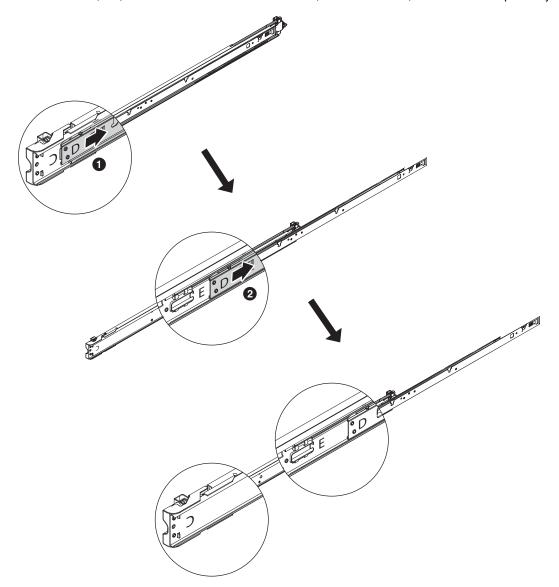
2. Install the mounting brackets onto to the corresponding rails using a T8 Torx screwdriver.
