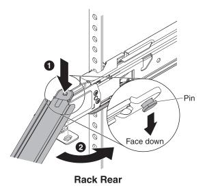
**3.** Connect the mounting bracket on the support bar to the outer mounting bracket on the rear of the rail.
