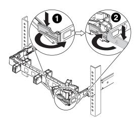
**6.** Attach the power cords and other cables to the rear of the server. Open the cable brackets on the CMA, route the cables, and then close the cable brackets.
