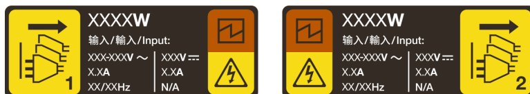
Figure 196. Example power supply unit label on the top cover
