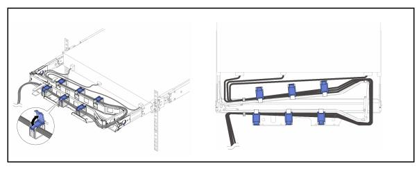
Step 2. Use the cable straps to tightly secure the cables to the front and rear of the CMA.
