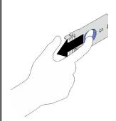
**Attention:** Release the mounting clip by pulling the ring-shaped release latch as illustrated.
