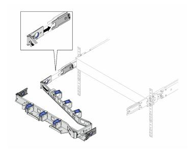
Step 2. Align two outer mounting clips with the outer tabs on the slides; then, push them until they snap into place.
