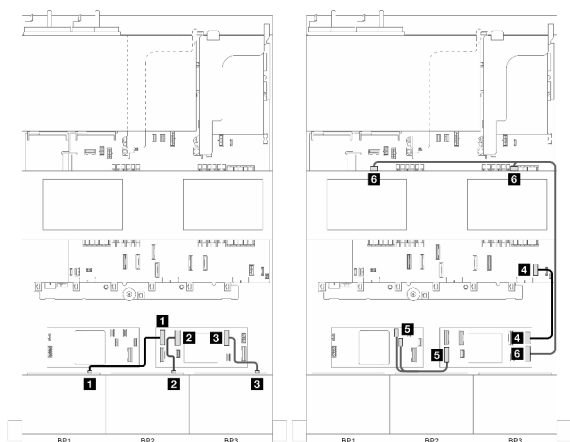
Figure 344. Signal cable routing part 1
