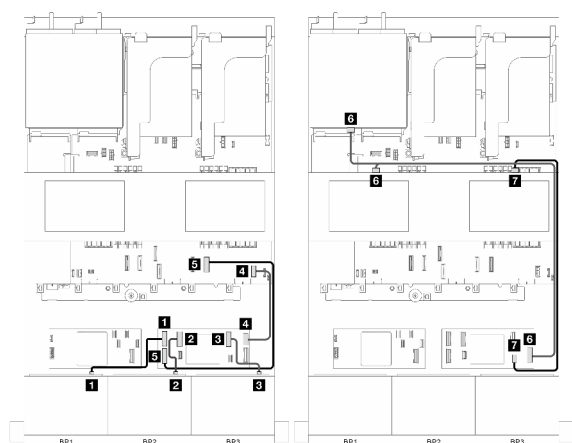
Figure 341. Signal cable routing part 1
