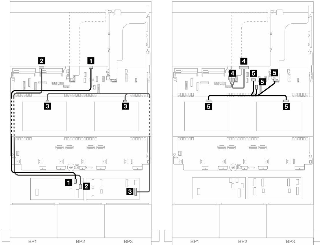
Figure 470. Middle/Rear backplane cable routing
