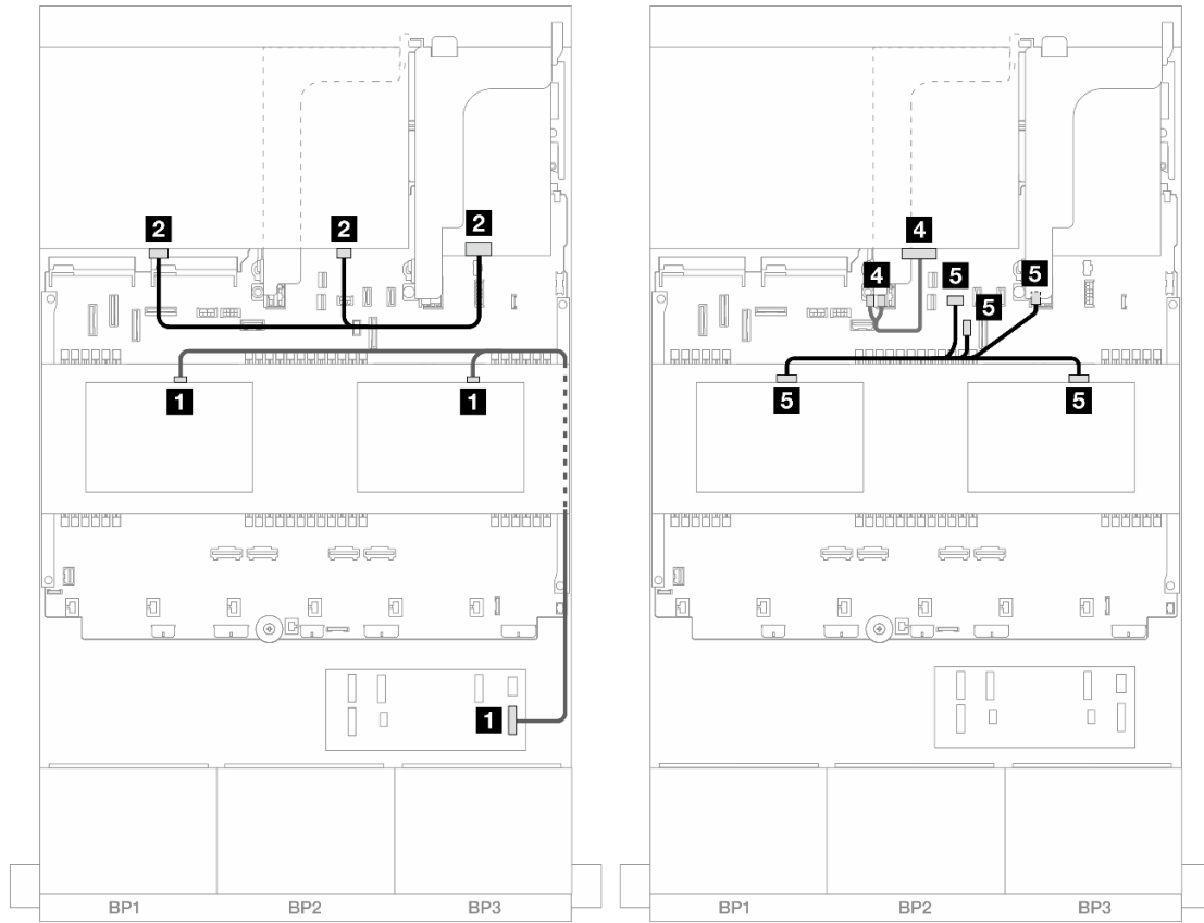
Figure 467. Middle/Rear backplane cable routing
