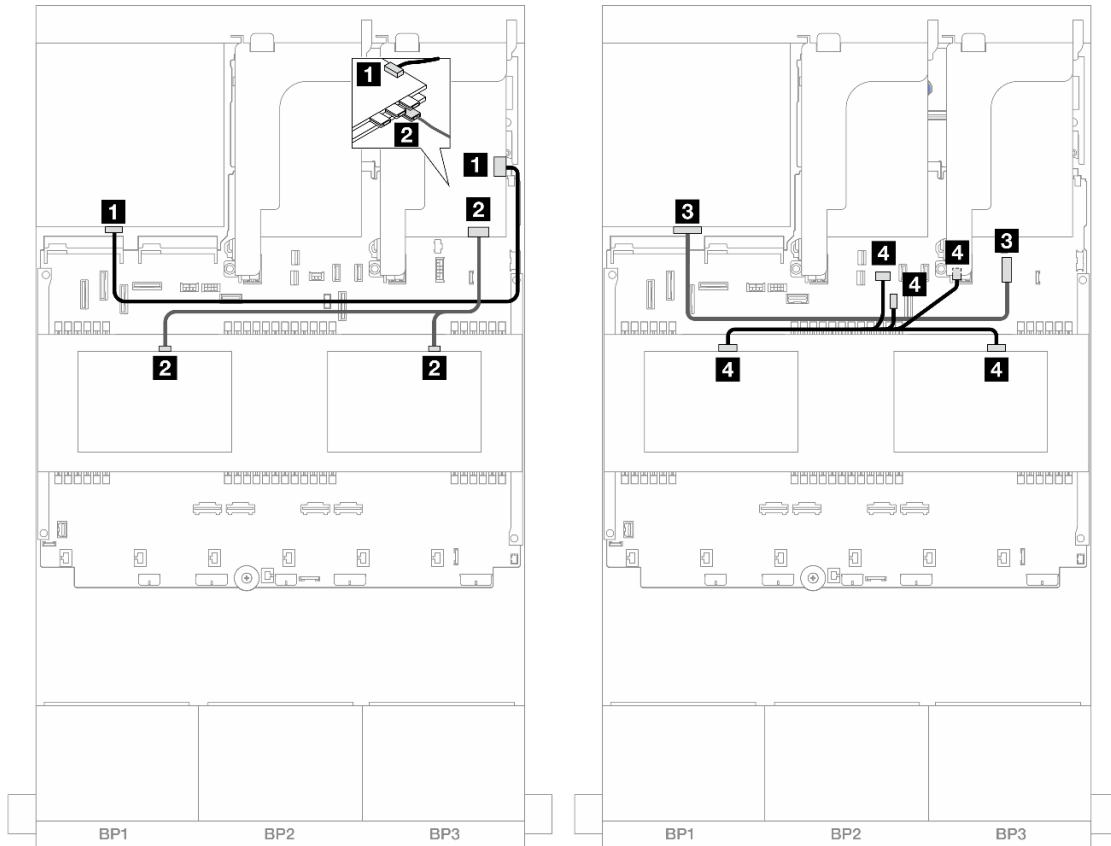
Figure 460. Middle/Rear backplane cable routing
