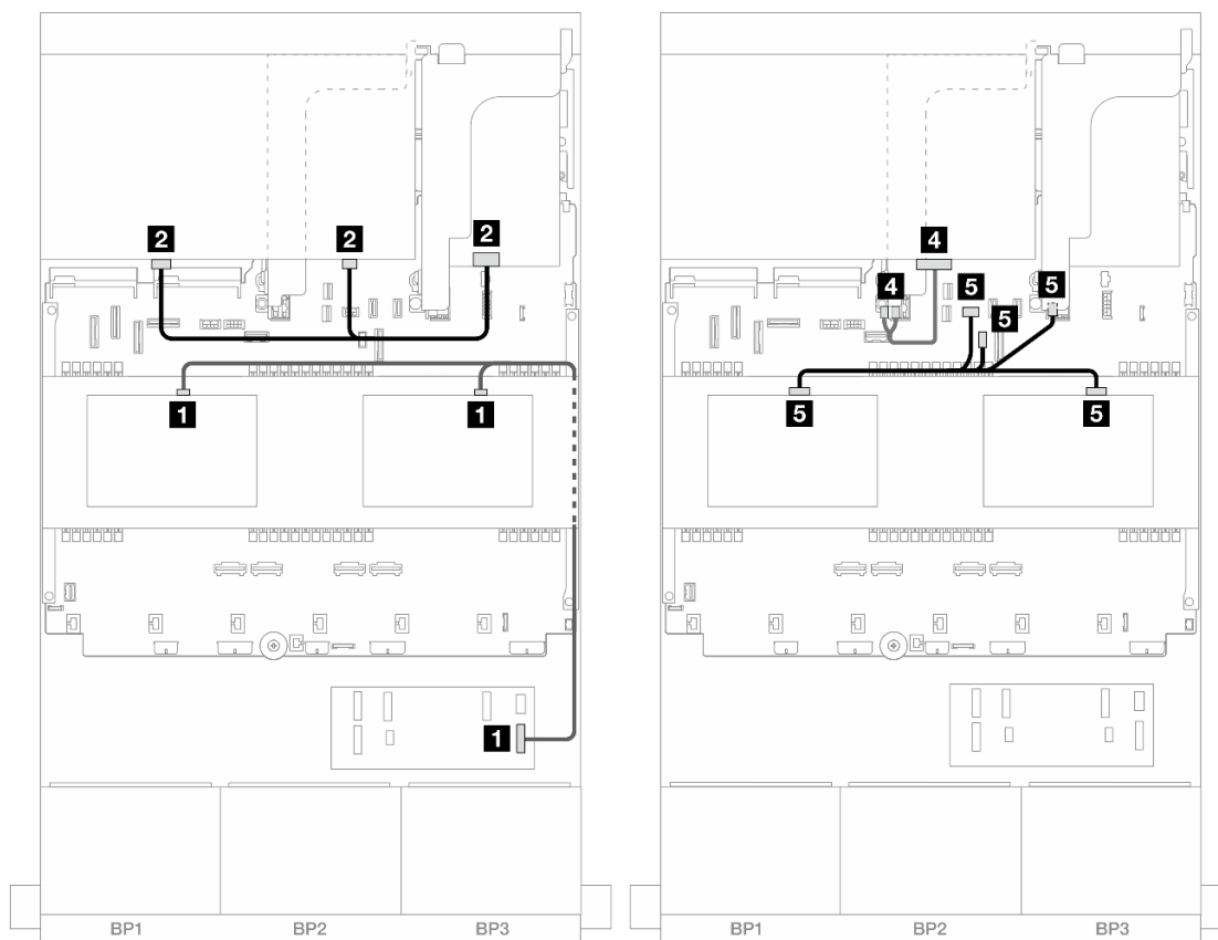
Figure 467. Middle/Rear backplane cable routing
