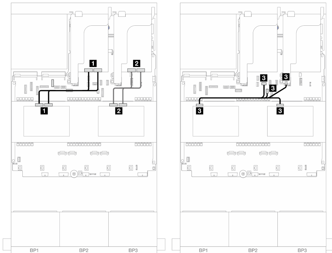
Figure 494. Middle backplane cable routing
