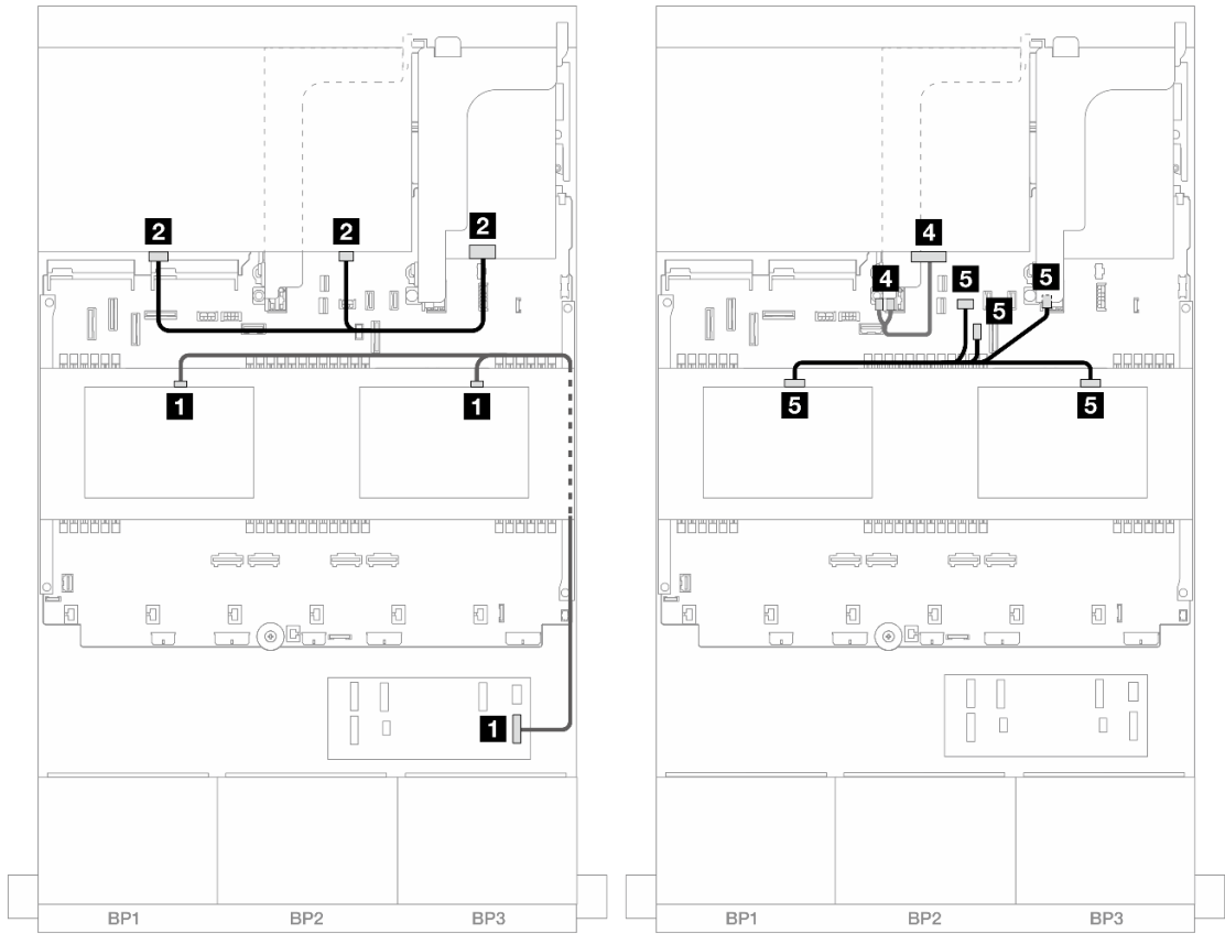
Figure 485. Middle/Rear backplane cable routing
