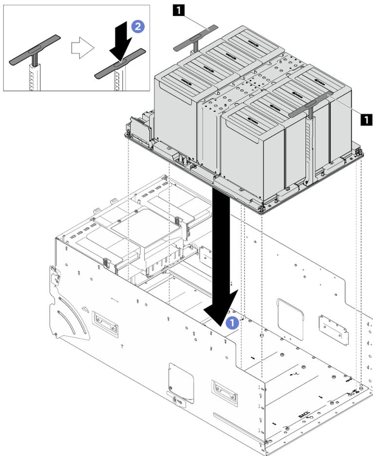
Figure 100. Installation du complexe GPU
