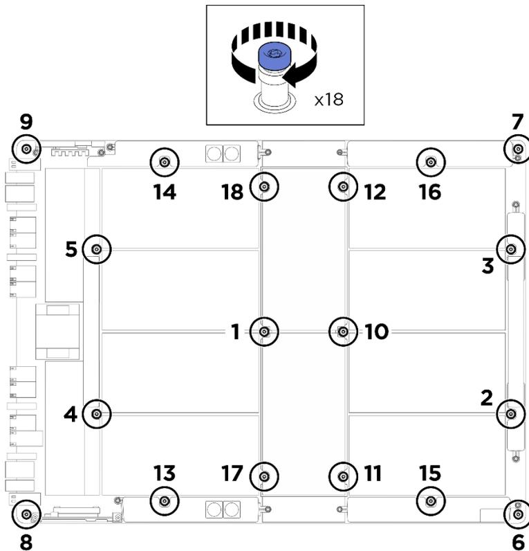
Figure 76. Installation des vis
