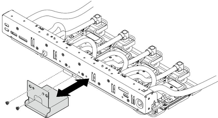
Figure 150. Installation du support de câble GPU
