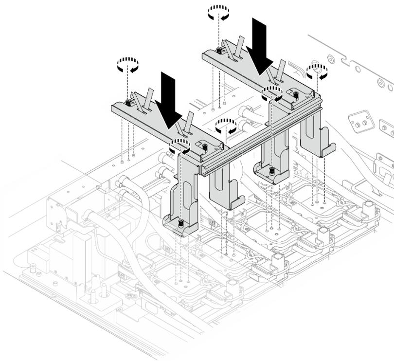
Figure 142. Installation des supports de transport
