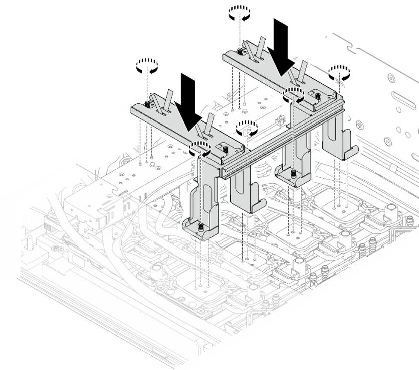
Figure 172. Installation des supports de transport
