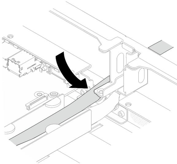
Figure 271. Installation du tuyau
