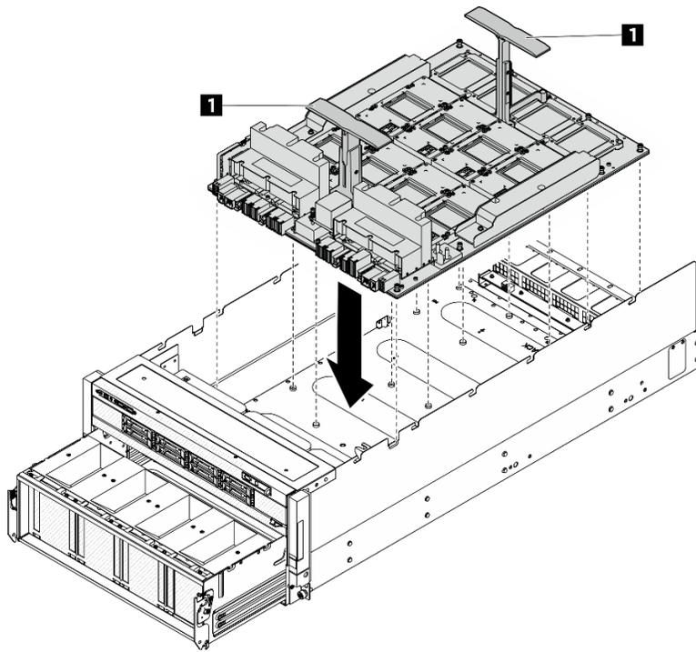
Figure 101. Installation du complexe GPU
