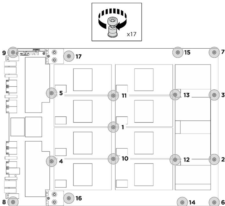
Figure 91. Installation des vis
