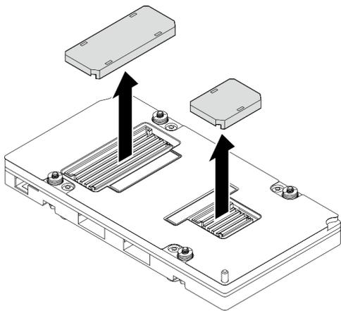
1. Para a GPU nova, remova as tampas do conector na parte inferior.
