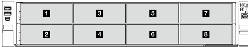
Figure 22. E3.S backplane numbering
