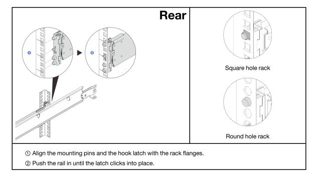
Step 1. Install the rear mounting pins to the rack.
