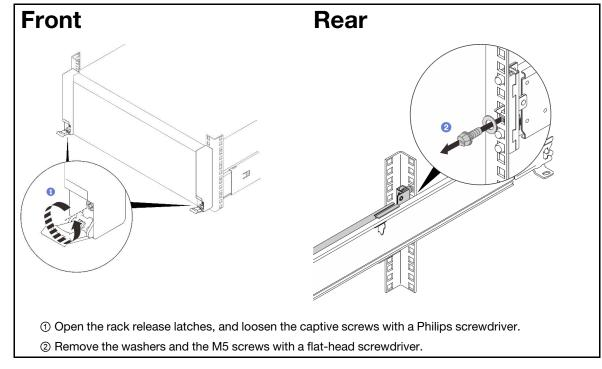
Step 1. Disengage the system if it has been secured to the rack.
