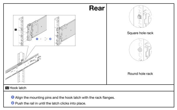
Step 2. Install the front mounting pins to the rack.
