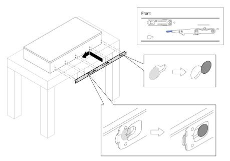
Step 4. Insert and tighten an M4 screw to secure the inner rail as shown.
