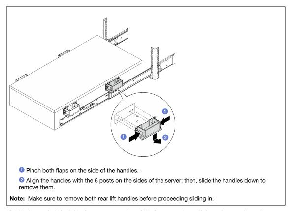
c. Lift the first pair of lock latches to proceed to slide the server in until the rails snap into place.
