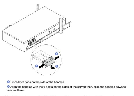
**Note:** Make sure to remove both front lift handles before proceeding to slide the server in.
