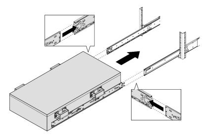
b. Remove the rear lift handles.
