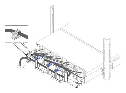
**Attention:** Carefully slide the server back and forward to ensure the cables do not pinch, bind, or hang down into the U space directly below the server.
