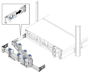
Step 2. Align two outer mounting clips with the outer tabs on the slides; then, push them until they snap into place.
