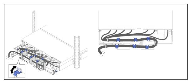
Step 2. Use the cable straps to tightly secure the cables to the front and rear of the CMA.
