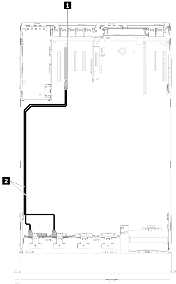
Figure 33. Cable routing, 8-bay backplane
