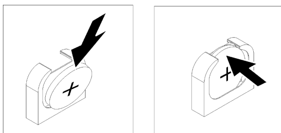
Figure 57. CMOS battery installation
