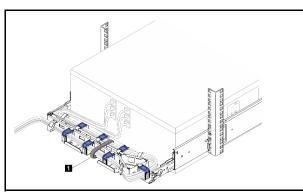
**Attention:** The long cable strap secures the CMA and cables in place during transportation. Unfasten the long cable strap before pulling the server out if the CMA is shipped with a rack.
