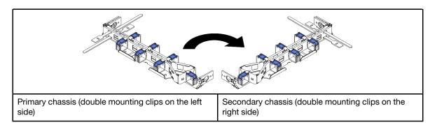
Step 2. Align the inner mounting clip with the inner tab on the slide; then, push it until it snaps into place.
