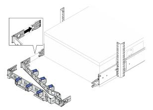
Step 3. Align two outer mounting clips with the outer tabs on the slides; then, push them until they snap into place.
